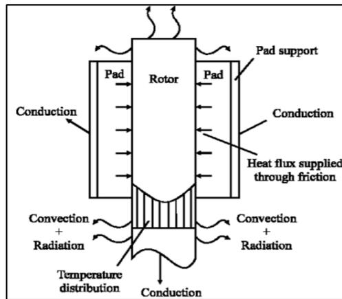
Fig 2. Modes of heat transfer in disc rotor [4]
