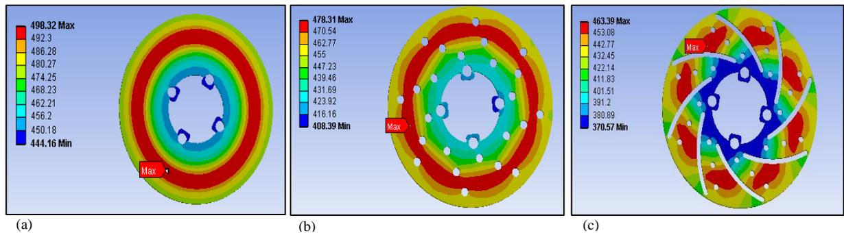
Fig 5. Temperature contours obtained in three rotors (in K); (a) Temperature contour on rotor 1; (b) Temperature contour on disc rotor 2; (c) Temperature contour on rotor 3
