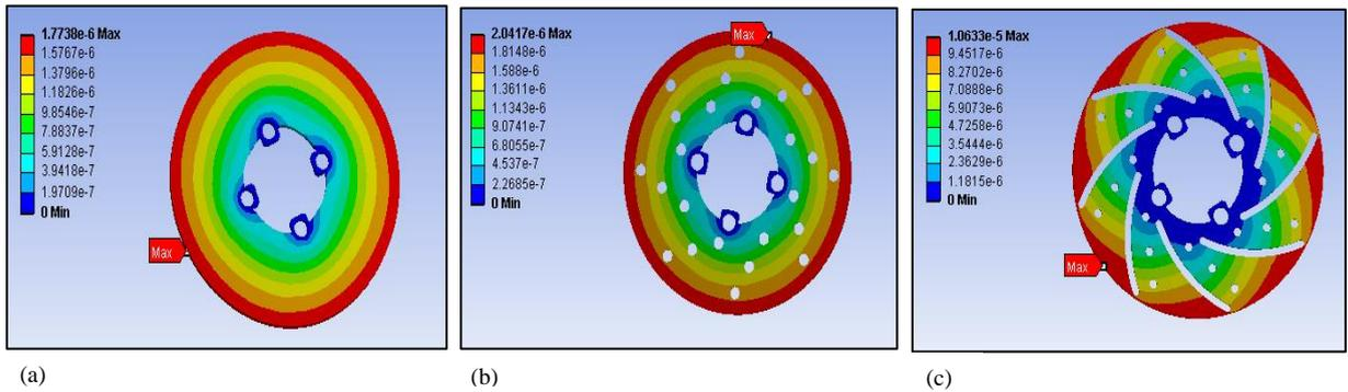
Fig 4. Total deformation plot in three rotors (in m); (a) Total deformation plot in rotor 1; (b) Total deformation plot in rotor 2; (c) Total deformation plot in rotor 3
