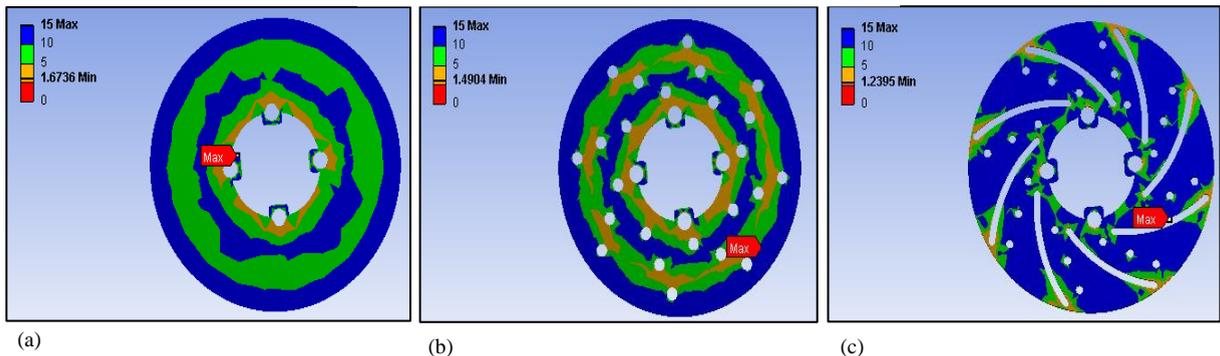
Fig 7. Fatigue factor of safety plot obtained in three rotors; (a) Fatigue factor of safety plot in rotor 1; (b) Fatigue factor of safety plot in rotor 2; (c) Fatigue factor of safety plot in rotor 3
