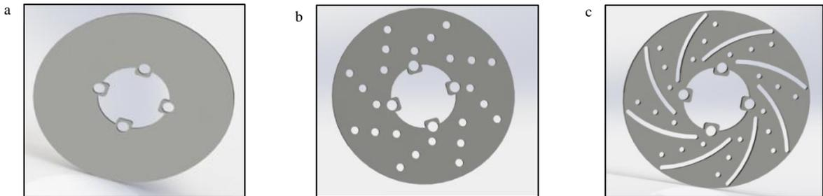
Fig 1. (a) Schematic model of disc rotor 1; (b) Schematic model of disc rotor 2; (c) Schematic model of disc rotor 3
