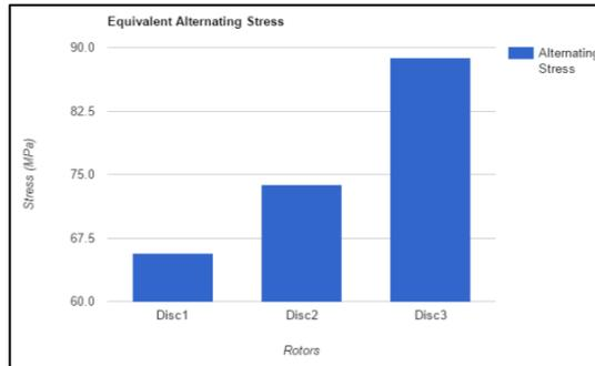
Fig 6. Equivalent alternate stresses induced in rotors
