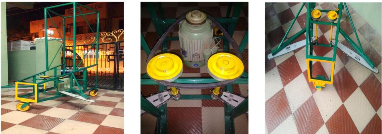
Figure 2. (a) Full view of the Harvesting Machine; (b) Motor and Pulley setup; (c) Blades used in the Machine
