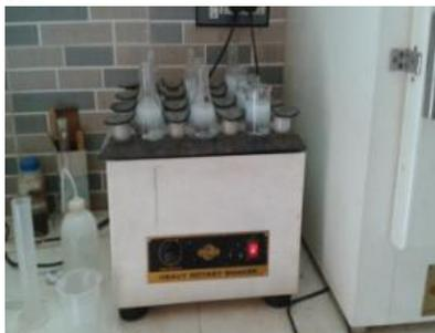
Fig. 2 Erlenmeyer flasks kept on heavy rotary stirrer
