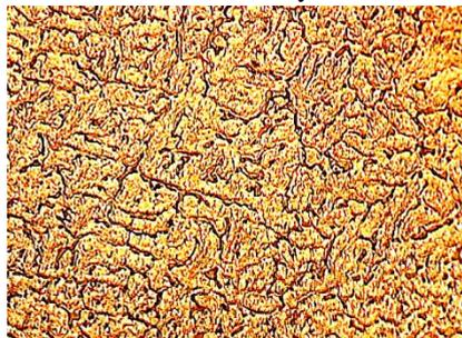
Fig. 3(a) Image of the microstructures of the Al–5-wt% Cu alloy
