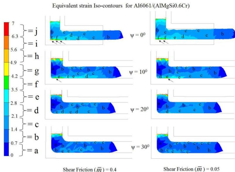
Fig.4. Equivalent Strain distribution at shear friction  $m=0.4$  and  $0.05$
