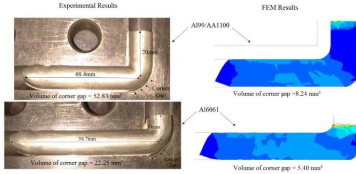
Fig.2: FE and experimental result comparison
