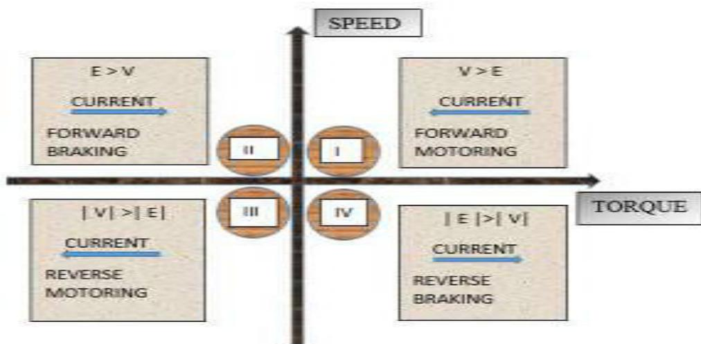
Fig.1. Four Quadrant Operation with Operating Modes.
