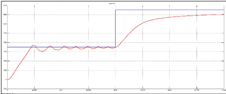
Fig.8. Output Speed Waveform of Proposed BLDC Motor Drive
