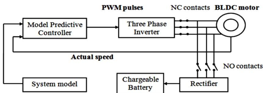
Fig.2. Block Diagram of Proposed System
