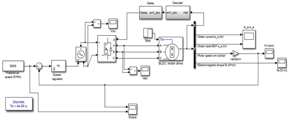
Fig.5. Simulink model of a conventional four quadrant control of BLDC motor.
