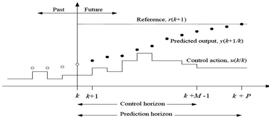
Fig.4. MPC Control Concept
