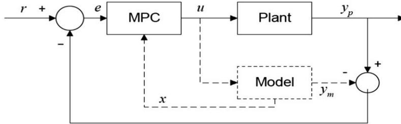
Fig.3. Block Diagram of MPC Technique
