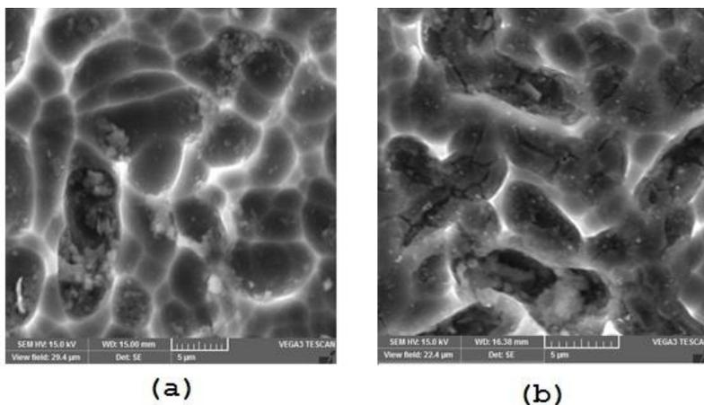
Fig. 4. (a) Polymer de-coated commercial Si solar cell (b) CNT-TiO<sub>2</sub>-coated Si - solar cell
