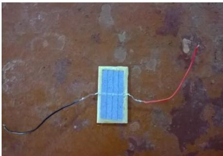
Fig. 3. CNT–Nano composite coated panel
