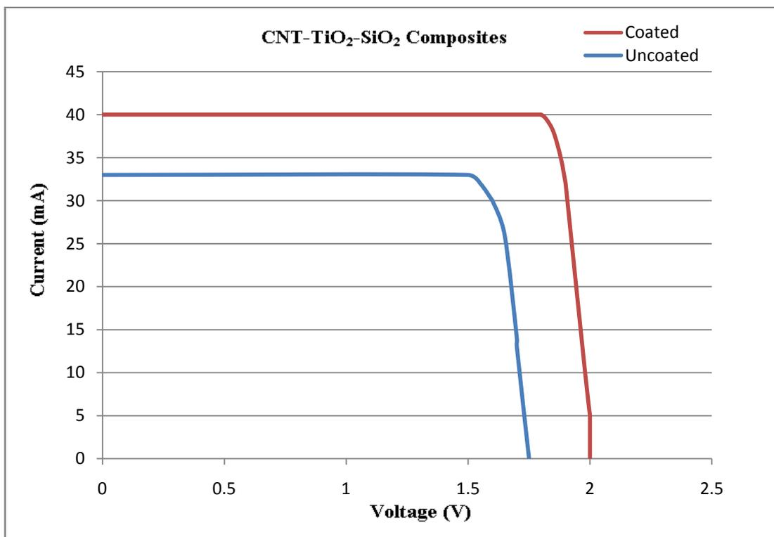
Fig. 5. I-V Curve for CNT coated cell
