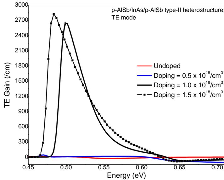
Fig. 3. TE optical gain in type-II p-AlSb/InAs/p-AlSb nano-scale heterostructure.
