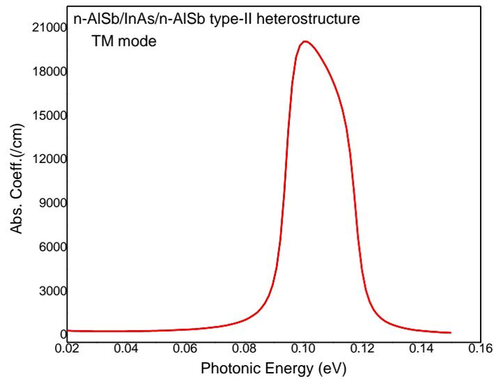
Fig. 1. Behaviour of absorption coefficient in n-AISb/InAs/n-AISb type-II nano-scale heterostructure.
