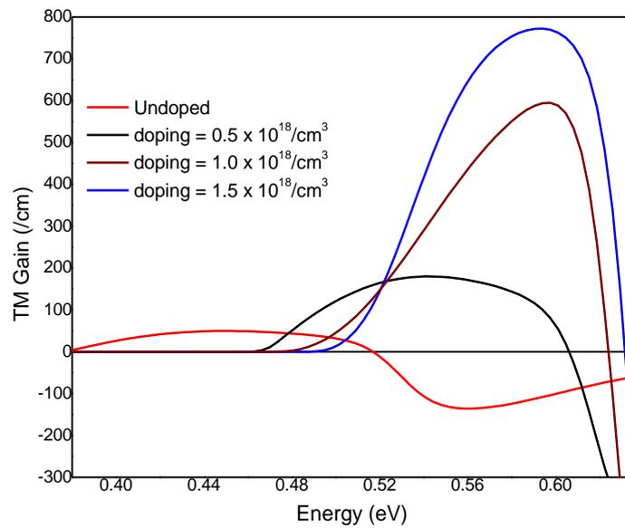
Fig. 2. TM optical gain in type-II p-AISb/InAs/p-AISb nano-scale heterostructure.
