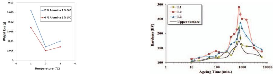
Fig.3 (a) The effect of age temperature on weight loss (b) Age hardening curves of composites - artificially aged at 180<sup>0</sup>C.
