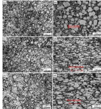
Fig.2 Microstructure of 7075 AMCs reinforced with nano sized SiC particles
