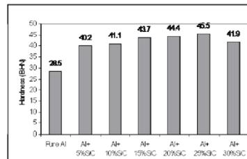
Fig. 1. Increase of Hardness with SiC Particulates
