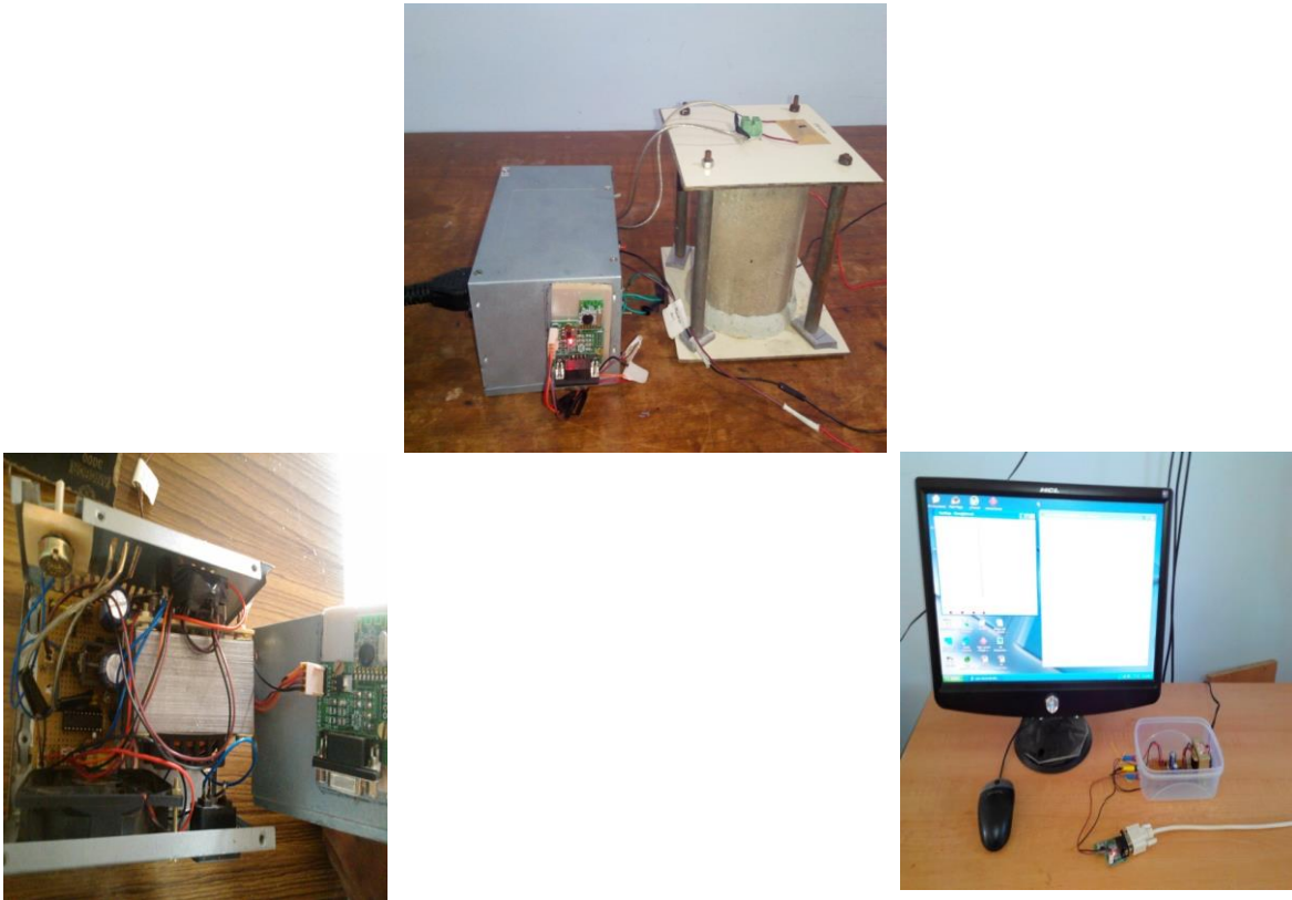
Fig. 5. Photograph of the fabricated hardware containing ZigBee, temperature sensor , and monitor view
