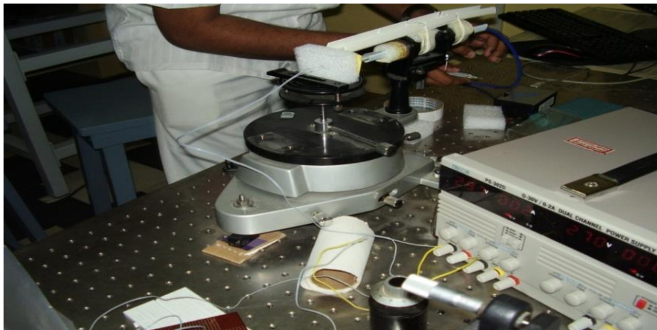
Fig. 8. Spectrometer setup used to record the spectra of LEDs
