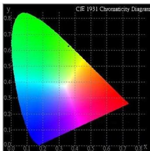
Figure 6: CIE Chromaticity diagram of  $\text{Er}^{3+}$  doped borosilicate glass of E specimen
