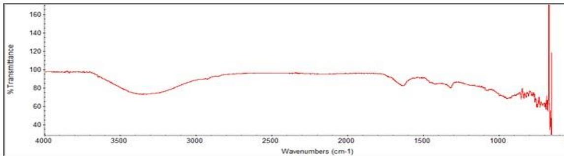
Figure 3: FTIR spectrum of  $\text{Er}^{3+}$  doped borosilicate glass of E specimen.
