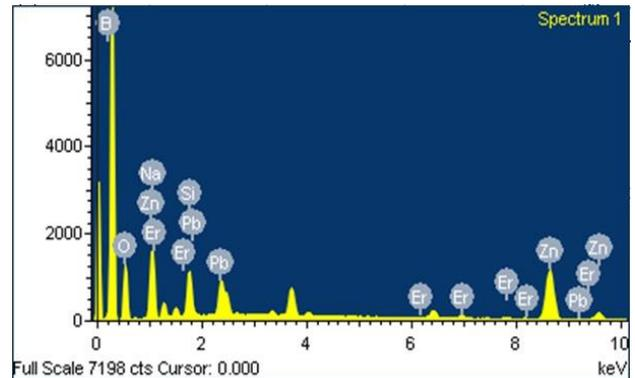
Figure 2: EDX spectrum of  $\text{Er}^{3+}$  doped borosilicate glass of E specimen.
