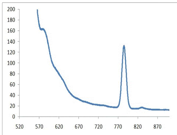
Figure 5: Fluorescence spectrum of  $\text{Er}^{3+}$  doped borosilicate glass of E specimen.
