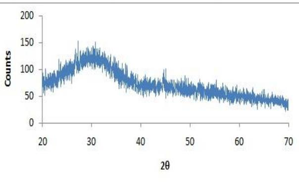
Figure 1: XRD spectrum of  $\text{Er}^{3+}$  doped borosilicate glass of E specimen.
