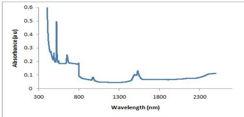
Figure 4: Absorption spectrum of Er<sup>3+</sup> doped borosilicate glass of E specimen.
