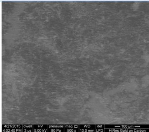
Figure 7: SEM image of Er<sup>3+</sup> doped borosilicate glass of E specimen.
