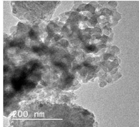
Figure 8: TEM image of Er<sup>3+</sup> doped borosilicate glass of E specimen.
