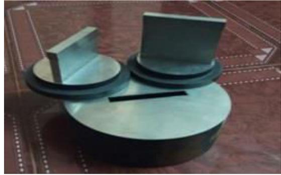
Fig 4(b) Finished Die and Punches
