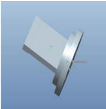
Fig. 2(a) 3D Model of Lower Punch
