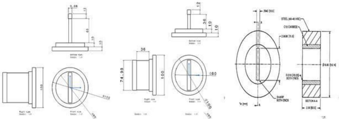
Fig.1 2D Design of Die and punches
