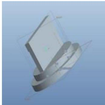
Fig. 2(b) 3D Model of Upper Punch
