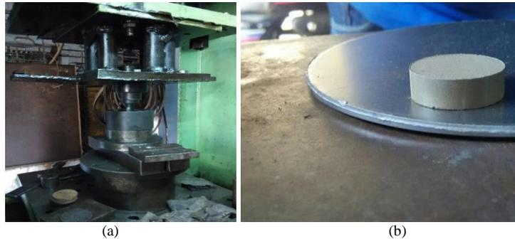
Fig. 3. (a) During compaction of compression specimen; (b) Compression after compaction
