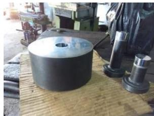
Fig. 2. Fabricated Compression Die
