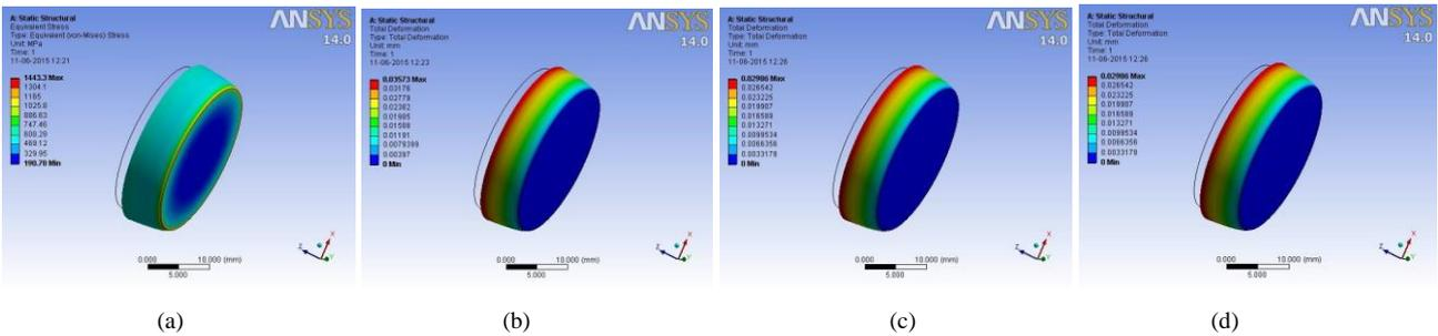
Fig. 6. (a) Pure iron- von-mises stress; (b) Pure iron- total deformation; (c) 0.25 wt.% CNT - von-mises stress; (d) 0.25 wt.% CNT – Total Deformation
