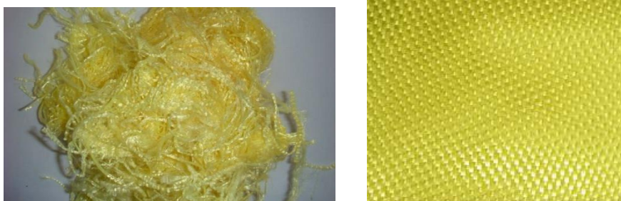
Figure 1. (a) Unprocessed Kevlar fibre; (b) Woven Kevlar fiber
