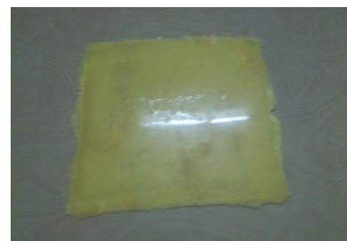
Figure 4. (a) Arrangement of Kevlar Composites; (b) Completed Kevlar composite
