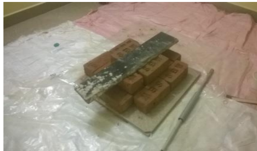
Figure 3. Weights placed on the Specimen
