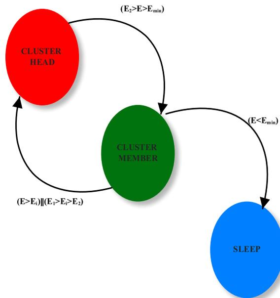
Fig. 2 Finite State Machine (FSM)
