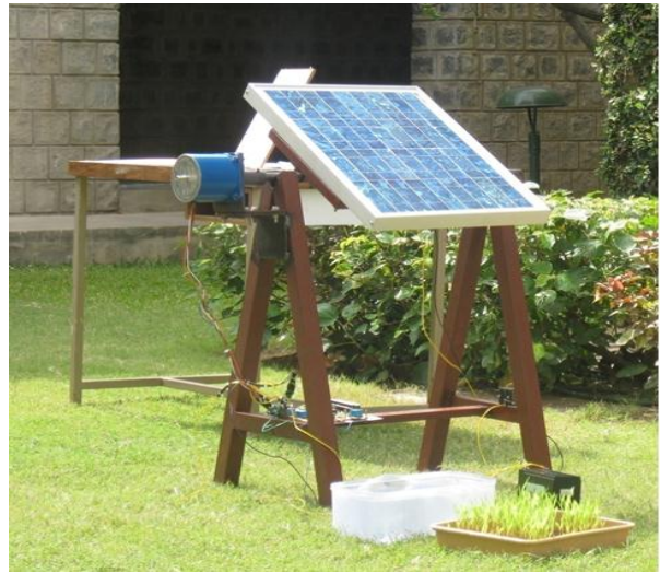
Fig 2 Sun Tracking PV System
