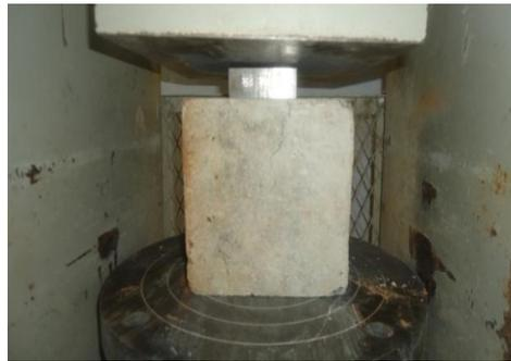
Fig. 7. Bearing strength test
