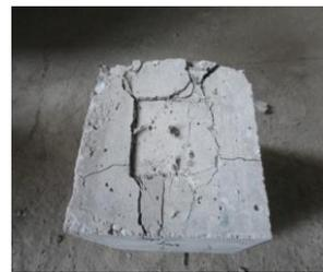
Fig. 9. Failure mode of cube under bearing loading
