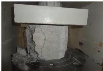
Fig. 8. Tested Cube under Compression loading
