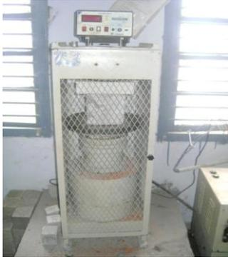
Fig. 6. Cube compressive test
