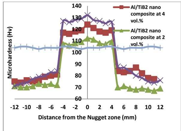
Fig. 4. Microhardness survey of Al/TiB<sub>2</sub> surface nano composites and as-received Al alloy
