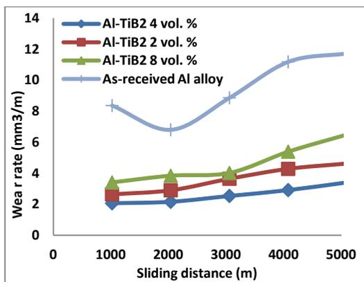
Fig.5. Wear rate of Al-TiB<sub>2</sub> surface nano composites and as-received Aluminum alloy
