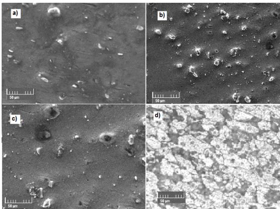
Fig. 3. SEM microstructures of Al/TiB<sub>2</sub> surface nano composites a) 2 vol. %, b) 4 vol. % and c) 8 vol. %
