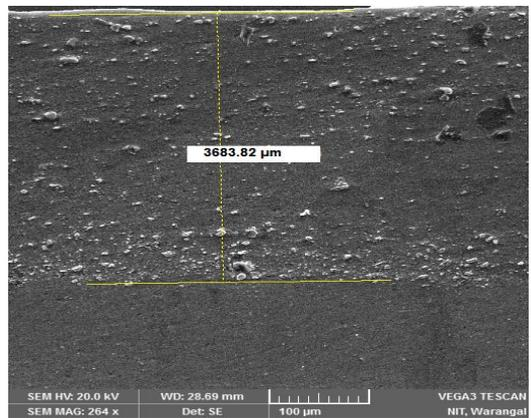
Fig.2. SEM image for depth of composite formed
