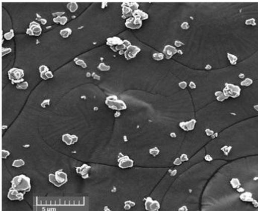
Fig.1. SEM micrographs of as-received TiB<sub>2</sub> particles
