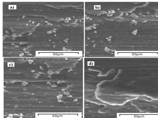
Fig.6. Wear morphology of Al-TiB<sub>2</sub> surface nano composites and as-received Aluminum
