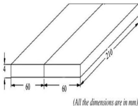
Fig.1. Schematic sketch of weld joint and tool
