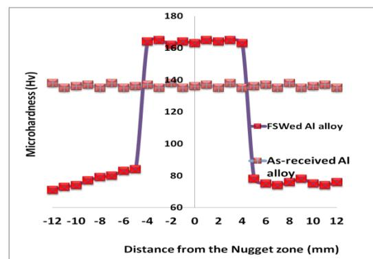
Fig.7. Hardness profiles evaluated across the weld nugget
