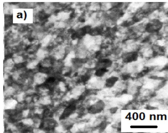
Fig.5. Microstructures of Aluminum alloy after FSW (Cryogenic cooling)
