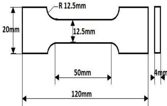
Fig.3. Schematic sketch of selection of samples for testing
