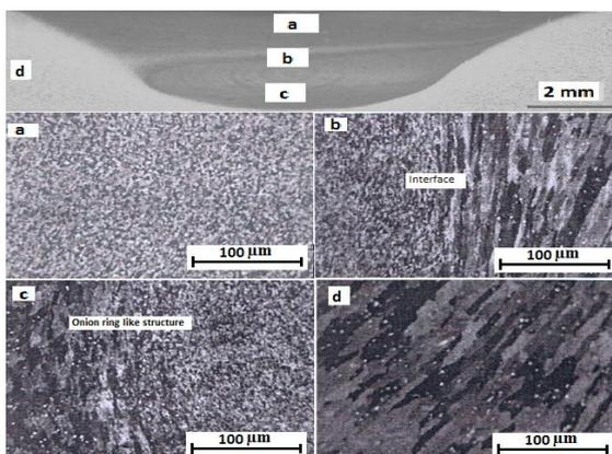
Fig.6. Microstructures of Aluminum alloy after FSW and Base material
