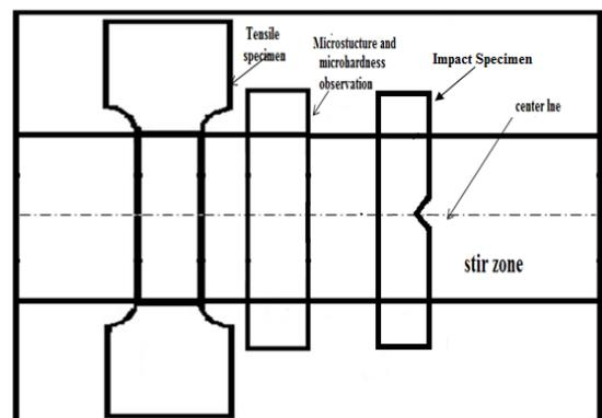
Fig.2. Schematic sketch of selection of samples for testing
