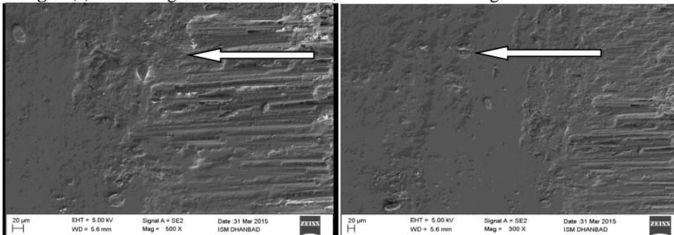
**Fig. 2 (f)** SEM image of wornout surface, oil-lubricated sliding at 3.14 m/s and 120 N.
