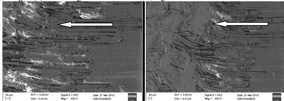
**Fig. 2 (i)** SEM image of wornout surface, argon medium at 3.14 m/s and 120 N.
