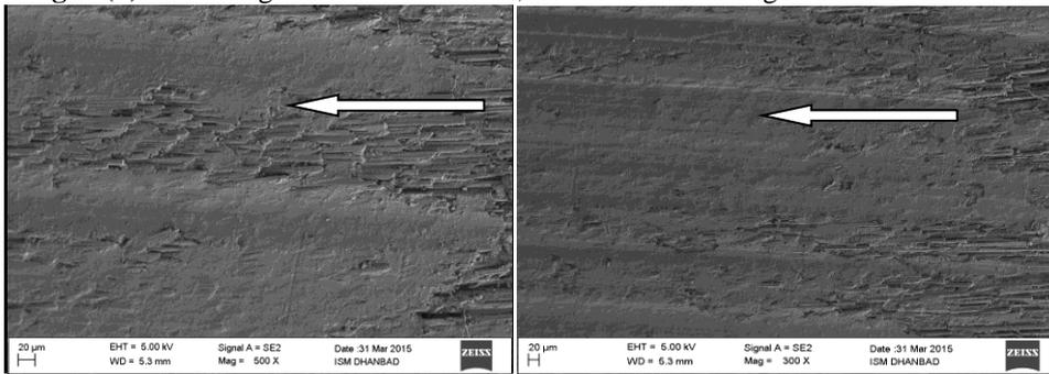
**Fig. 2 (e)** SEM image of wornout surface, oil-lubricated sliding at 3.14 m/s and 80 N.
