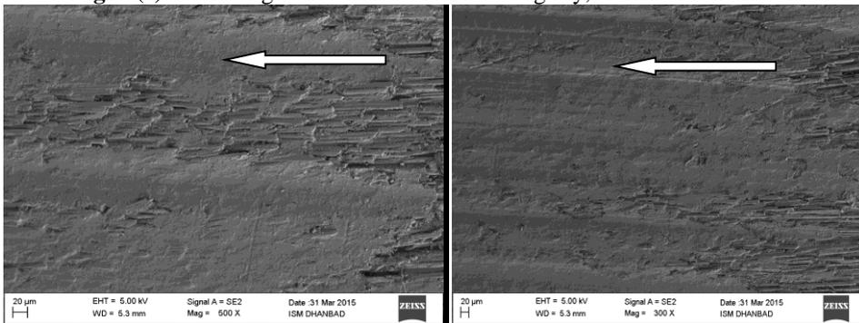
**Fig. 2 (d)** SEM image of wornout surface, oil-lubricated sliding at 3.14 m/s and 40 N.
