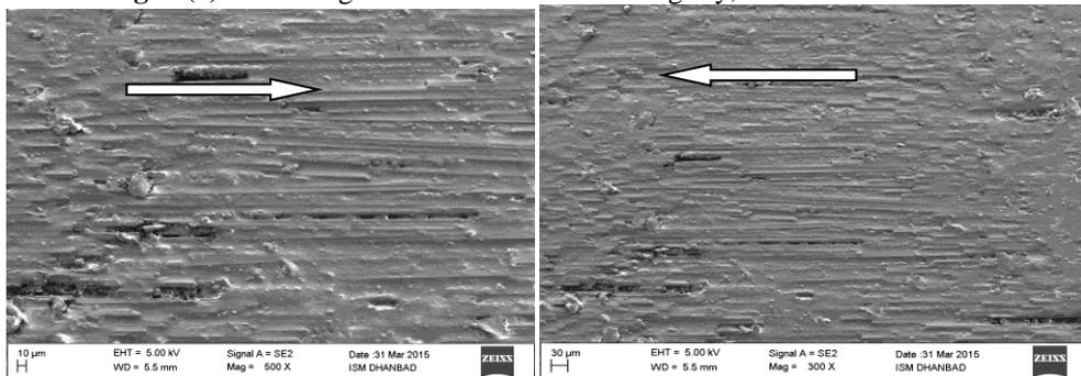
**Fig. 2 (b)** SEM image of wornout surface sliding dry, at 3.14 m/s and 80 N..
