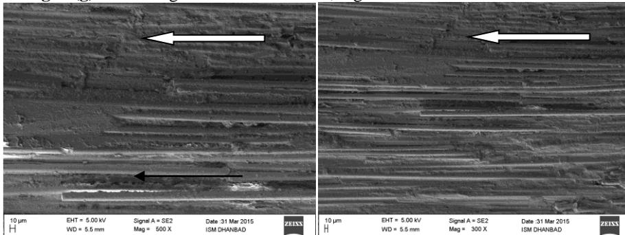
**Fig. 2 (h)** SEM image of wornout surface, argon medium at 3.14 m/s and 80 N.
