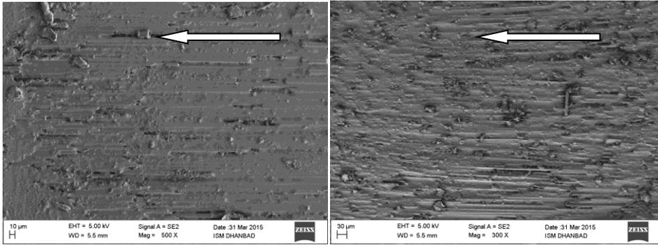
**Fig. 2 (c)** SEM image of wornout surface sliding dry, at 3.14 m/s and 120 N.
