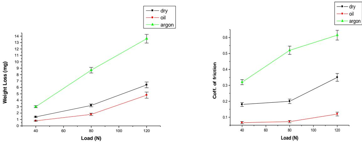
**Fig. 1 (a)** Weight loss v/s Load and Coefficient of friction v/s Load for CFRP, sliding under all three environmental conditions at 2.51 m/s and 1508 m.
