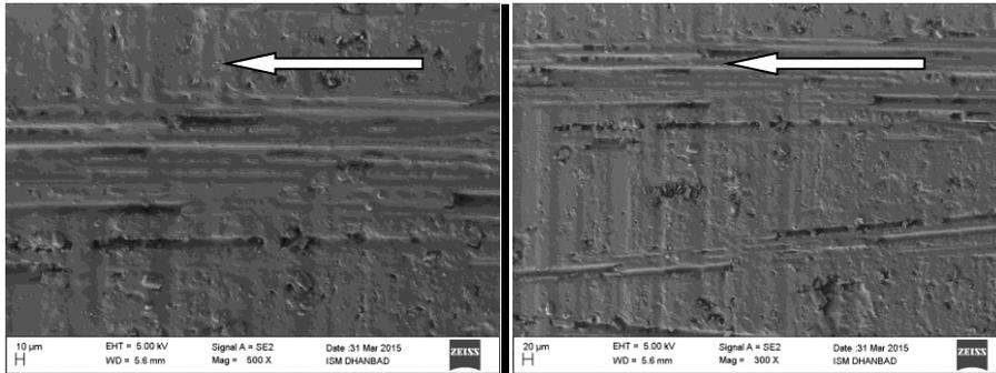
**Fig. 2 (g)** SEM image of wornout surface, argon medium at 3.14 m/s and 40 N.
