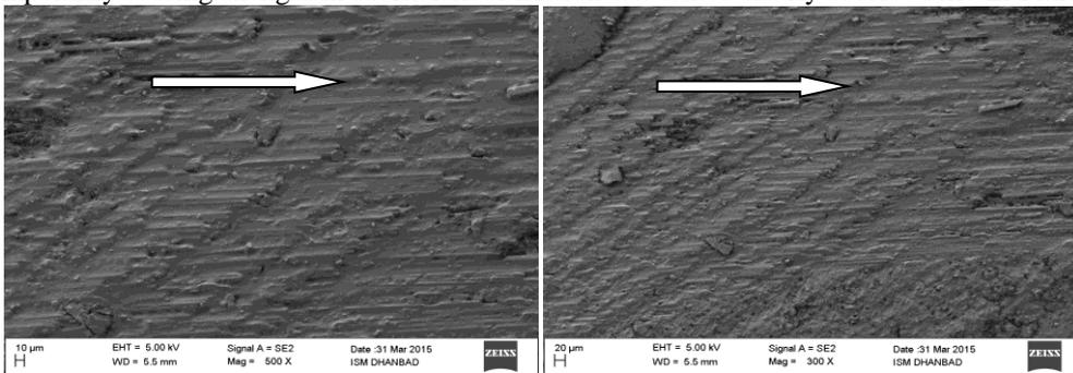
**Fig. 2 (a)** SEM image of wornout surface sliding dry, at 3.14 m/s and 40N.
