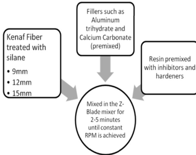
Fig. 1. Mixing Methodology for the Bulk Molding Compound.
