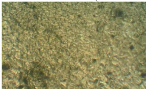
Fig 3.3.1. Micro Structure at 910rpm and feed 30mm/min
