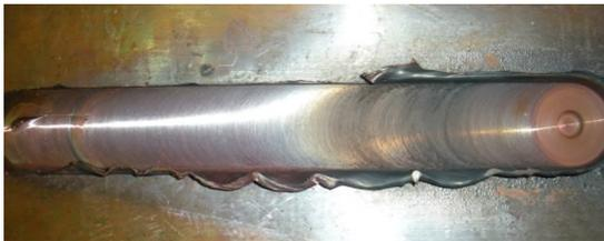
Figure 2.2.1 Welded copper Plate at condition 1
