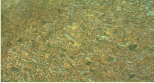
Fig 3.3.3 Micro Structure at 910 rpm and feed 30mm/min sic used
