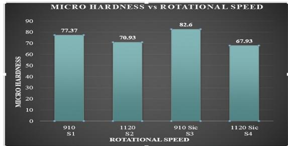
Graph 3.2.2(c) Hardness by varying the Tool Speed
