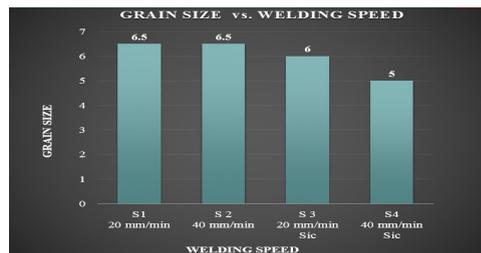
Graph 3.3(a) Grain size vs. Welding Speed
