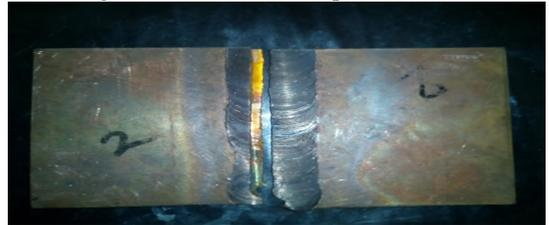
Figure 2.2.2 Welded cu plate at condition 2
