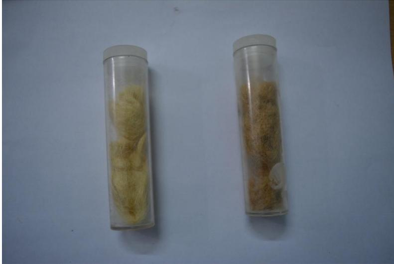
**Fig. 1(a)**  $H_2O_2$  treated jute fiber **(b)** Untreated jute fiber
