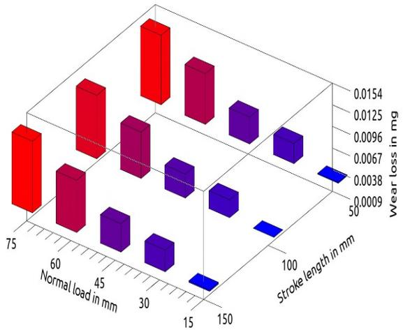
Fig. 5. Wear loss vs Stroke length vs Normal load plot for a 7% Silicon alloy, 400 m sliding and average velocity of 0.4 m/s
