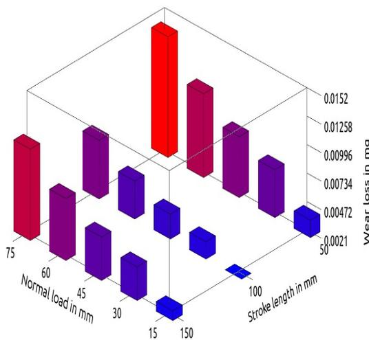
Fig. 6. Wear loss vs Stroke length vs Normal load plot for a 13% Silicon alloy, 400 m sliding and average velocity of 0.4 m/s
