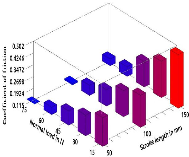
Fig. 4. CoF vs Stroke length vs Normal load plot for a 18% Silicon alloy, 400 m sliding and average velocity of 0.4 m/s
