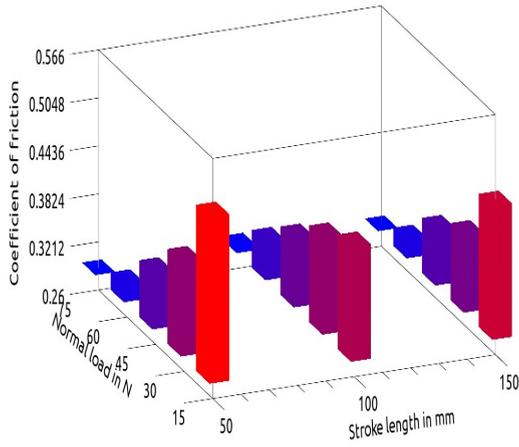
Fig. 2. CoF vs Stroke length vs Normal load plot for a 7% Silicon alloy, 400 m sliding and average velocity of 0.4 m/s
