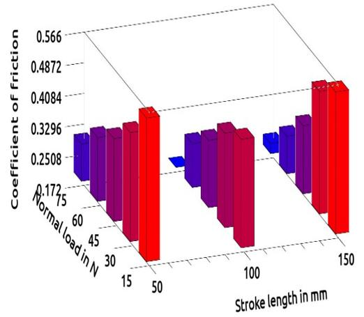
Fig. 3. CoF vs Stroke length vs Normal load plot for a 13% Silicon alloy, 400 m sliding and average velocity of 0.4 m/s
