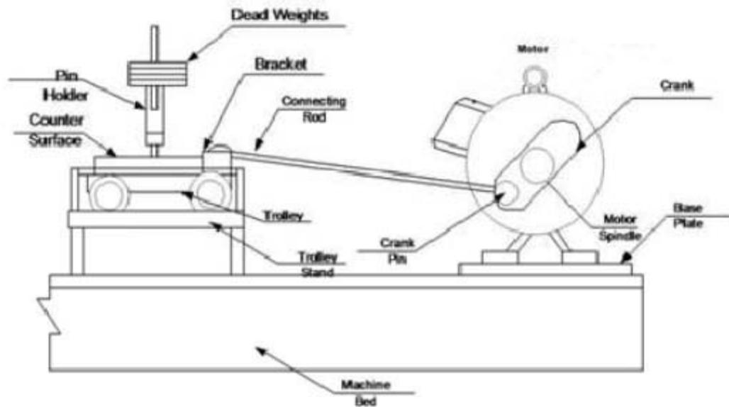
Fig. 1. Schematic Diagram of Reciprocating Wear Test Rig.
