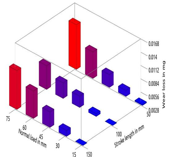
Fig. 7. Wear loss vs Stroke length vs Normal load plot for a 18% Silicon alloy, 400 m sliding and average velocity of 0.4 m/s
