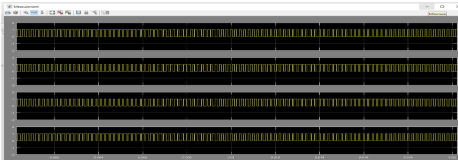
Figure 10: SPWM based gating pulses for VSI
