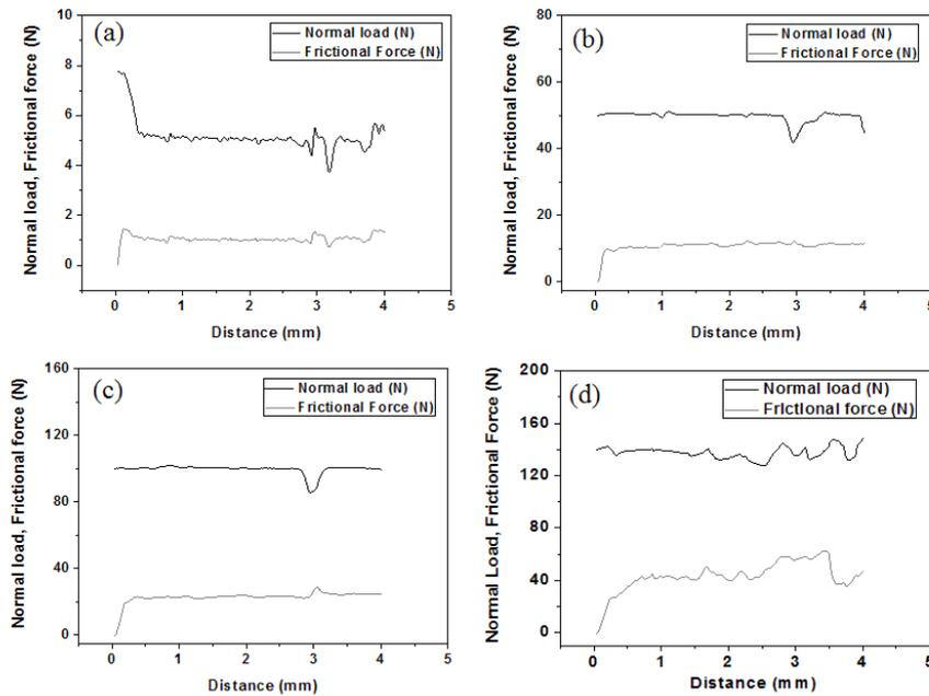
Fig. 2. Normal load and frictional force versus distance graphs for conventionally brazed joint at a normal load of (a) 5 N, (b) 50 N, (c) 100 N and (d) 140 N.
