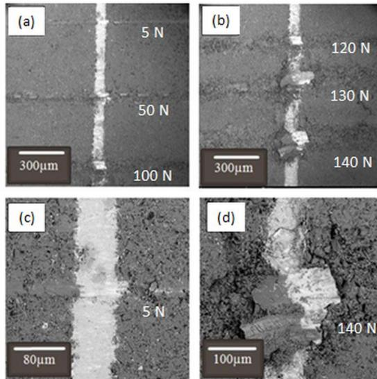
Fig. 5. (a) SEM images showing scratch tracks for microwave brazed joint at a normal load of (a) 5 N, (b) 50 N, (c) 100 N and (d) 140 N.
