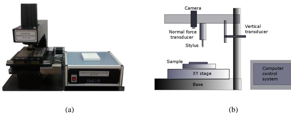
Fig. 1. (a) Scratch tester and (b) schematic diagram of scratch tester.
