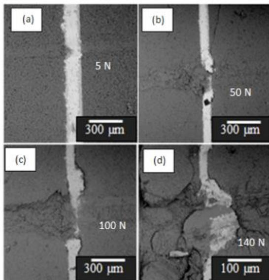
Fig. 3. SEM images showing scratch tracks for conventionally brazed joint at a normal load of (a) 5 N, (b) 50 N, (c) 100 N and (d) 140 N.
