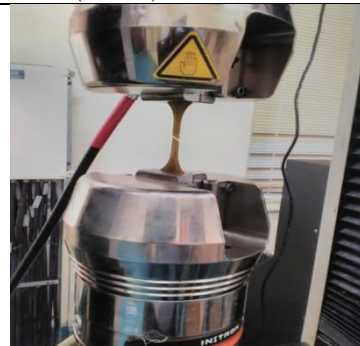
Fig. 5 Specimen after fracture on universal testing machine (INSTRON 4507)
