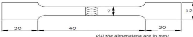
Fig. 4. Dimensions of tensile specimen.
