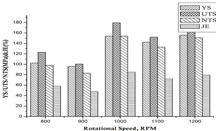
Fig. 5. Effect of rotational speed on tensile properties.
