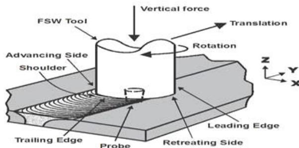
Fig. 1. Schematic representation of FSW principle.
