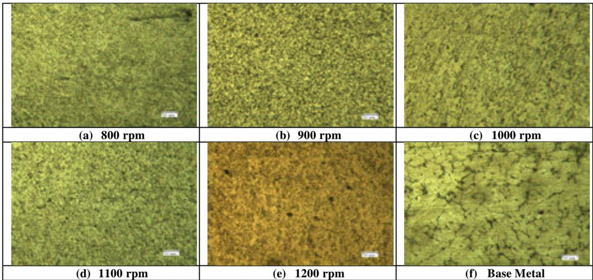
Fig.6. Effect of rotational speed on FSP (Nugget) zone microstructure. (a) 800RPPM, (c) 900RPM, (b) 1000RPM, (d) 1100RPM, (e) 1200RPM (f) Base metal
