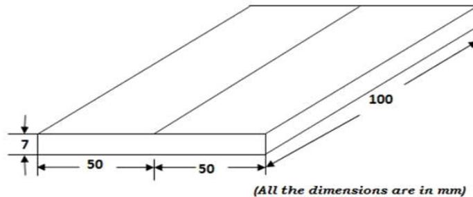
Fig. 3. Dimensions of square butt joint.
