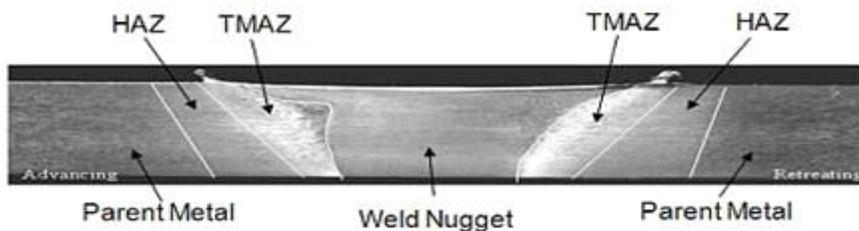
Fig. 2. Different regions of FSW joint.
