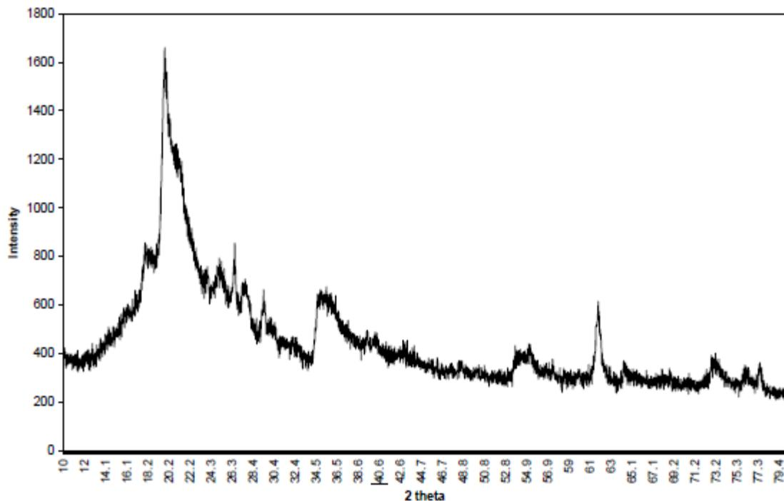
Fig. 5. XRD diffractogram of LDPE ( (Supri A.G 2008) [14]
