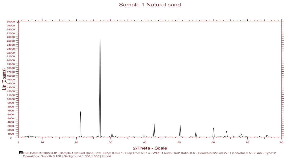
Fig.. 1 Typical graph of microfines x-ray diffraction analysis (ICAR-107)
