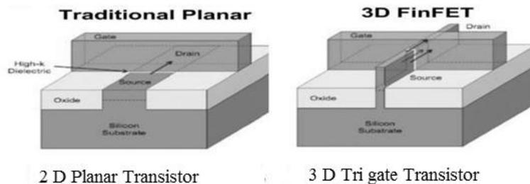
Fig 1: Structure of FinFET
