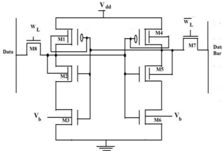
Fig: 3 Proposed SRAM cell
