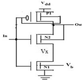
Fig: 2 Modified Schmitt Trigger
