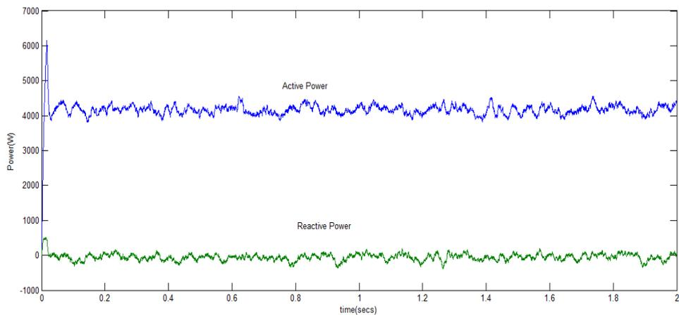
Fig 6 Reactive power and Active power provided by three phase source
