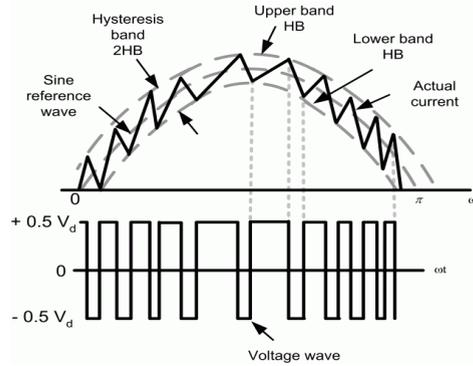
Fig 5 Hysteresis Current control waveform
