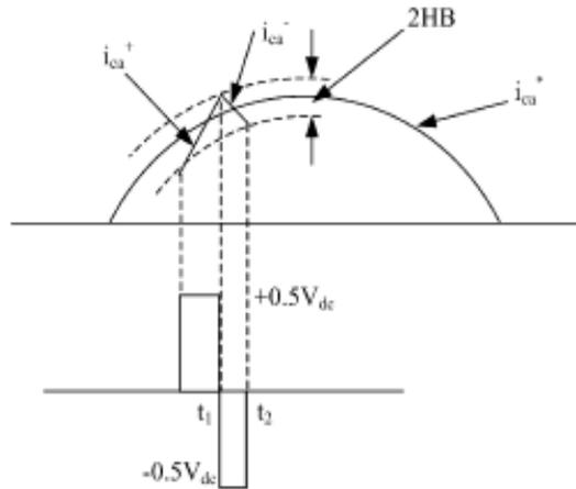
Fig. 6 Current and voltage waveform with adaptive hysteresis band current control
