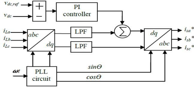
Fig 4 Block diagram of conventional SRF method
