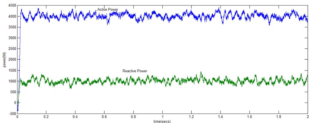
Fig 7 Reactive power and active power supplied by PV generation system
