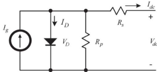
Fig 2. Equivalent circuit of a PV cell
