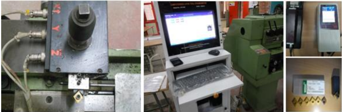
Figure 1. The experimental set inclusive of lathe tool dynamometer, data acquisition, surface roughness tester, inserts and tool holder.
