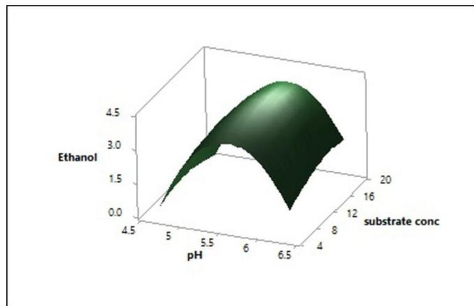
Fig. 3. Surface plots showing effect of substrate concentration and pH on ethanol concentration
