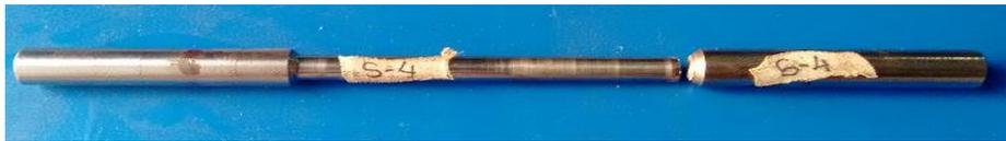
Fig. 1 Failed specimen tested on fatigue testing machine
