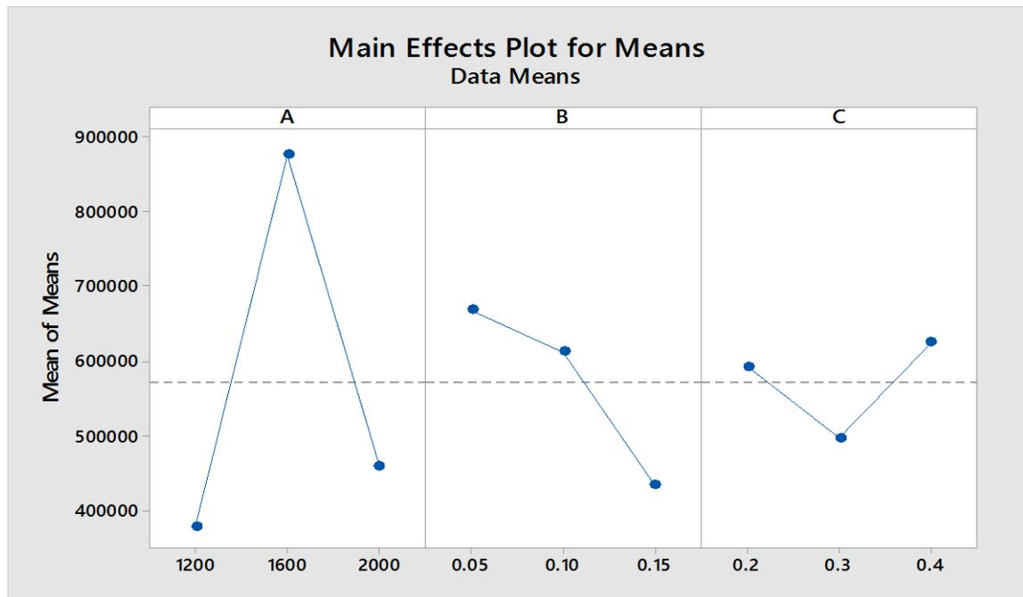
Fig. 4 (A) Mean of Means for cutting speed, (B) Mean of Means for feed rate, (C) Mean of Means for depth of cut.
