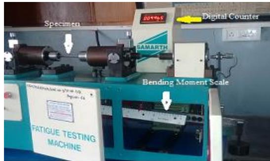
Fig 1. Bending Rotating Fatigue testing machine
