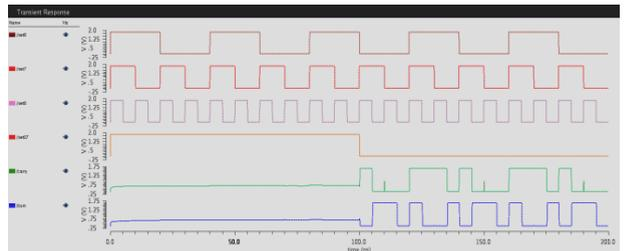
Fig 10: Simulation results of body-biased PG hybrid full adder
