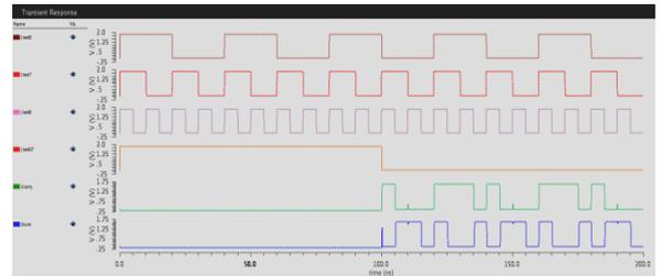
Fig 16: Simulation results of body-biased HS-DFPH hybrid full adder
