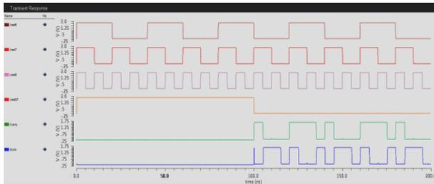
Fig 15: Simulation results of body-biased HS-DHPF hybrid full adder
