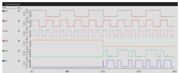
Fig 13: Simulation results of body-biased HS-DG hybrid full adder
