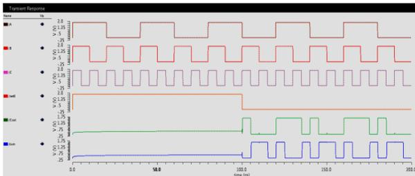
Fig 9: Simulation results of body-biased DG hybrid full adder
