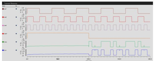
Fig 12: Simulation results of body-biased DFPH hybrid full adder
