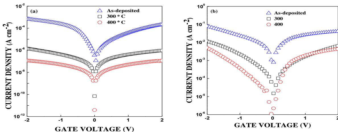
Figure 5: Current-Voltage characteristics of (a) Ge and (b) Si devices
