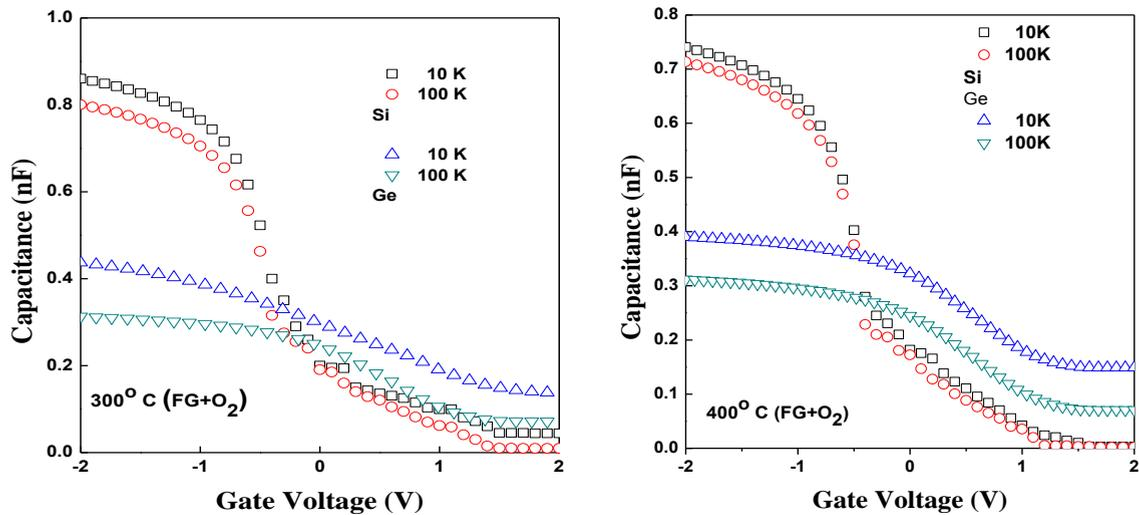
Figure 4: C-V characteristics of annealed at Ge- and Si- MOS devices
