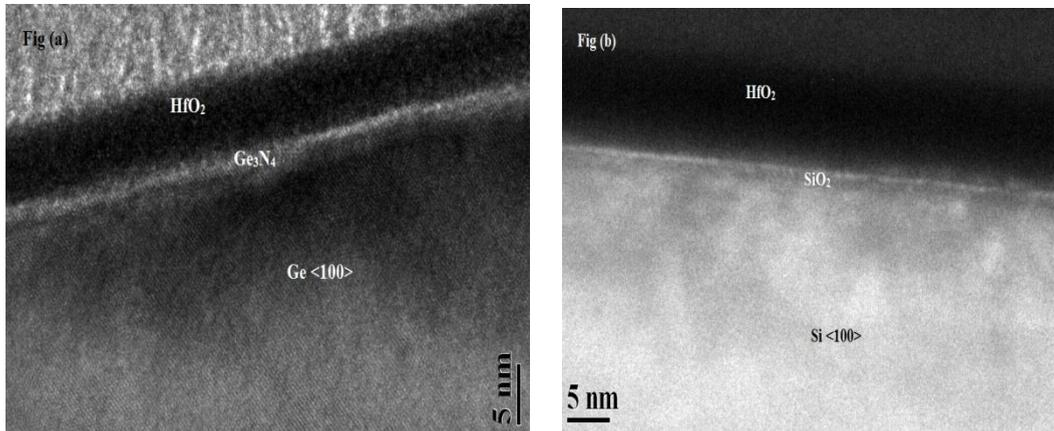
Figure 2: HREM images taken from (a) Ge devices and (b) Si devices before annealing
