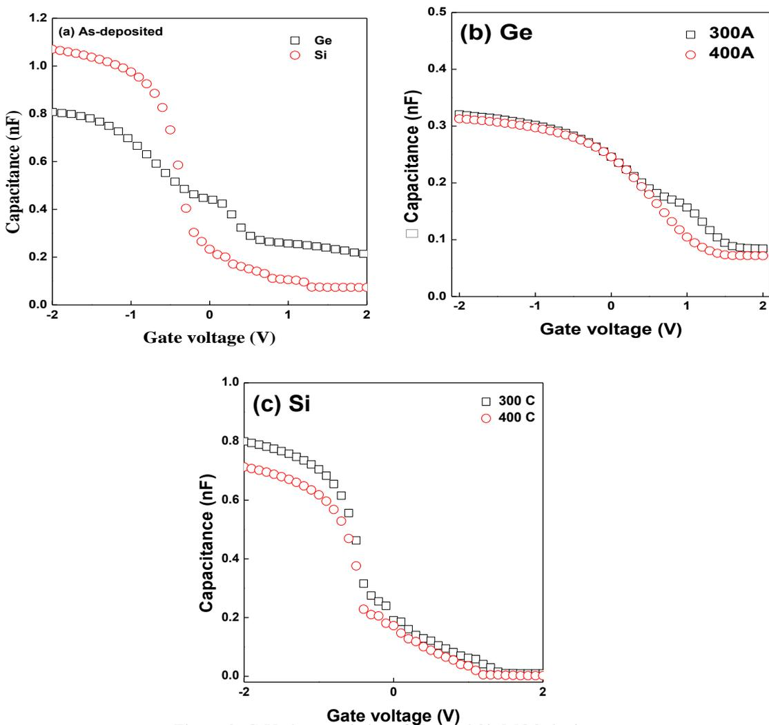
Figure 3: C-V characteristics of Ge- and Si- MOS devices
