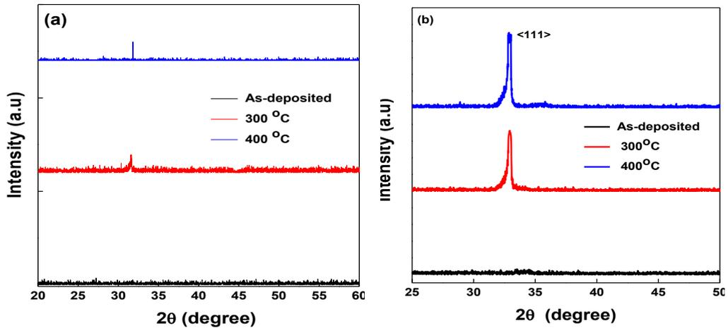
Figure 1: X-Ray Diffraction Spectra of (a) Ge (b) Si devices
