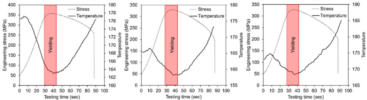
Fig. 7. Yielding identification from stress and temperature data by passing electric current through 0 (left), 45 (center), 90°(right) rolling direction samples
