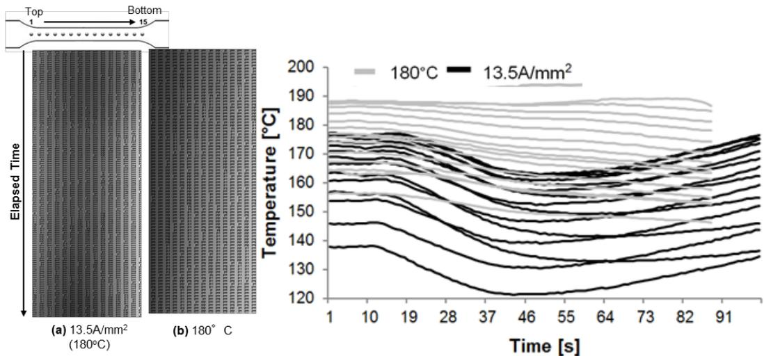
Fig. 4. Left: Temperature pattern on samples throughout deformation: 13.5A/mm<sup>2</sup>, 180° C (black shade is hotter region) [24] and Right: Differences in thermal behavior between thermal and electrical conditions (0° to roll direction) [24]
