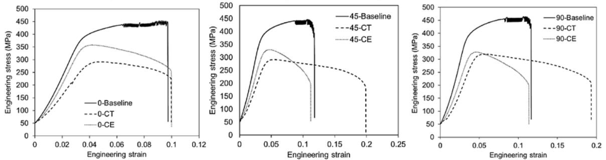
Fig. 3. Engineering stress-strain curve in 0 (left), 45 (center) and 90°(right) to rolling direction (CT – Continuous Temperature; and CE – Continuous Electricity)
