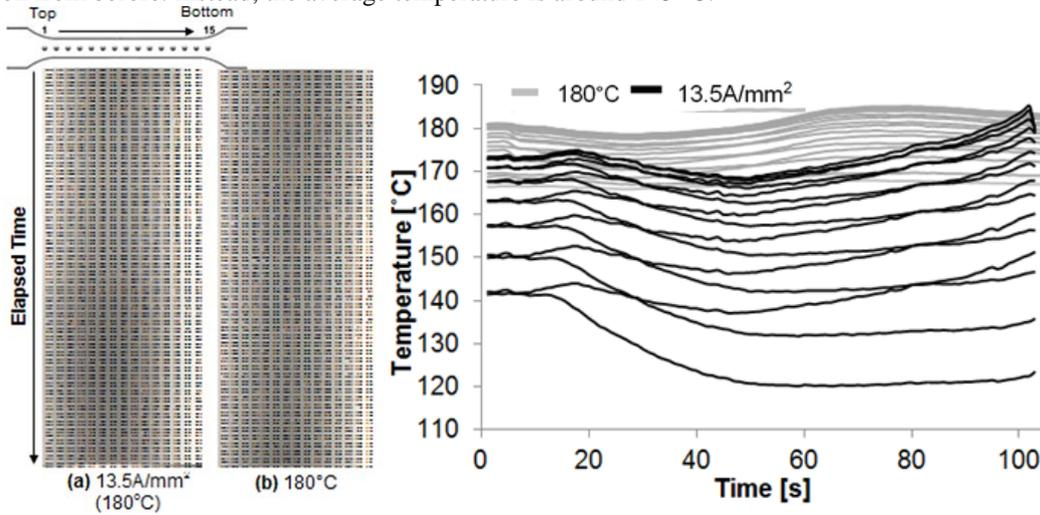
Fig. 6. Left: Temperature of samples throughout deformation: 13.5A/mm2, 180°C and Right: Differences in thermal behavior between thermal and electrical conditions (90° to roll direction)
