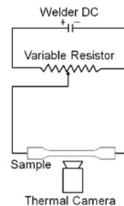
Fig. 2. Welder circuit setup for experiments [23-24]
