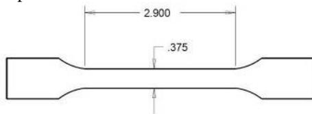
Fig. 1. Specimen Dimensions [23-24]
