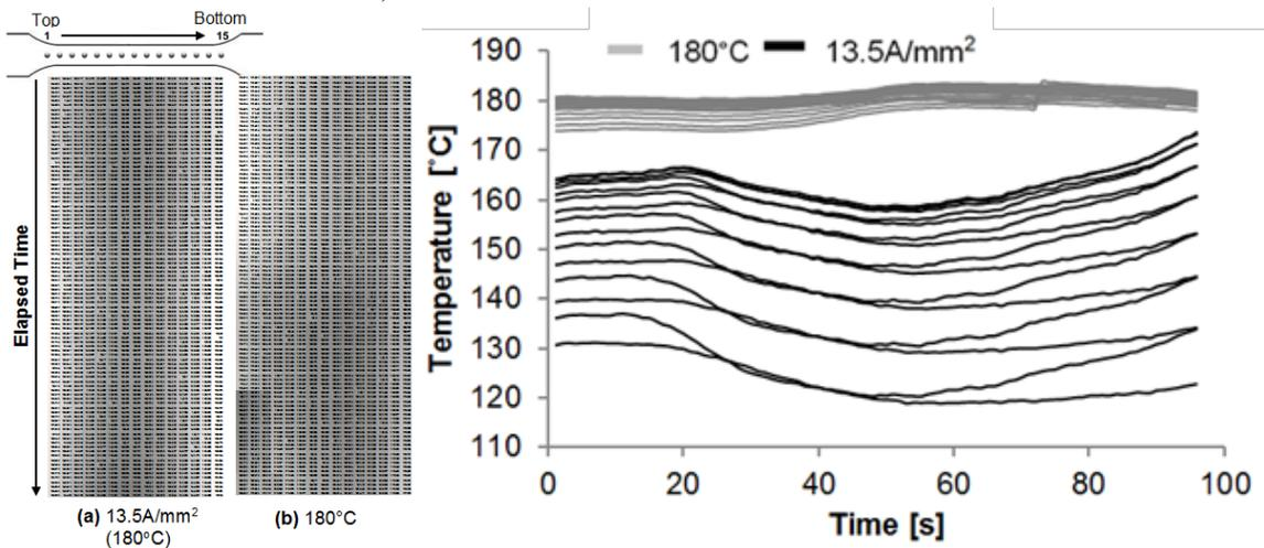
Fig. 5. Left: Temperature pattern on samples throughout deformation: 13.5A/mm<sup>2</sup>, 180°C and Right: Differences in thermal behavior between thermal and electrical conditions (45° to roll direction)
