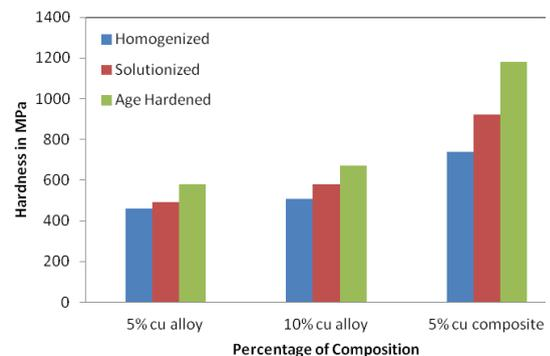
Figure 10 Hardness values of the alloys and composite under various heat-treatment conditions
