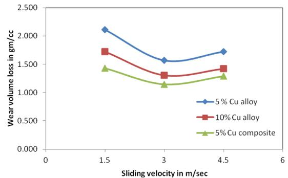
Figure 8 wear volume loss versus sliding velocity of alloys and composite
