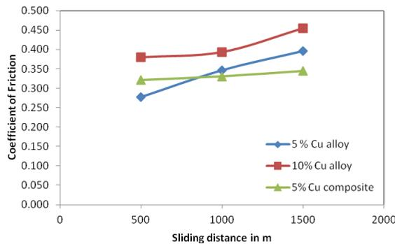
Figure 13 coefficient of friction versus sliding distance of alloys and composite
