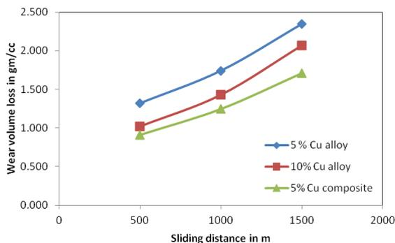
Figure 9 wear volume loss versus sliding distance of alloys and composite
