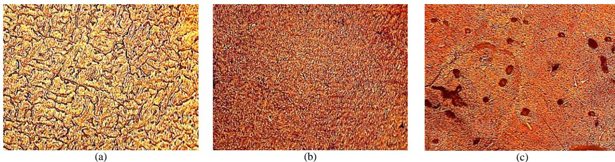
Figure 2 Images of the microstructures of the (a) Al-5-wt% Cu alloy, (b) Al-10-wt% Cu alloy, and (c) Al-Cu composite.
