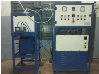
Figure 1 Electric resistance furnace used for manufacturing of alloys and composite
