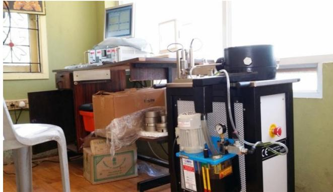
Figure 6 pin-on-disc equipment used for wear testing
