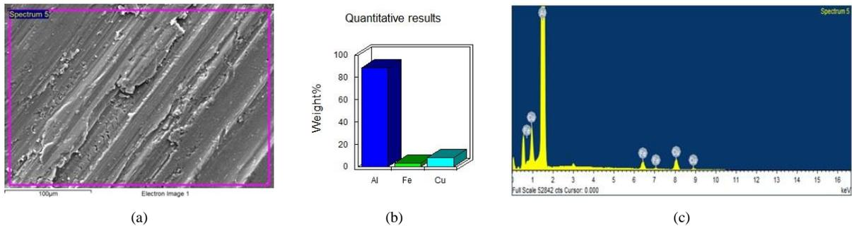
Figure 14 (a) SEM micrograph of worn surface of Al-5-wt% Cu alloy, (b) its quantitative results and (c) its corresponding EDAX analysis
