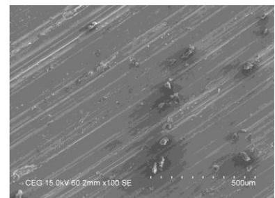
Figure 17 SEM image of worn out pin of Al-Cu composite at 30 N load, 1.5 m/sec sliding velocity and 1500 m sliding distance
