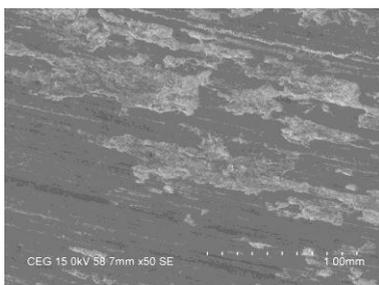
Figure 15 SEM image of worn out pin of Al-5-wt% Cu alloy at 10 N load, 4.5 m/sec sliding velocity and 1500 m sliding distance
