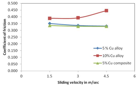
Figure 12 coefficient of friction versus sliding velocity of alloys and composite
