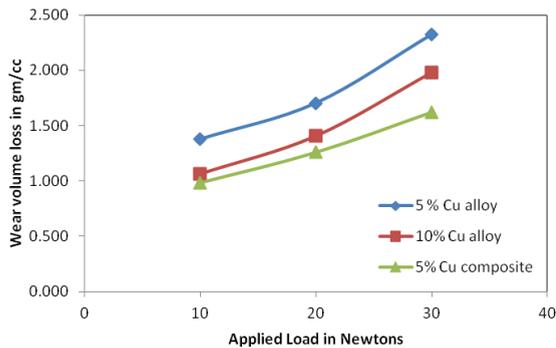
Figure 7 wear volume loss versus load of alloys and composite
