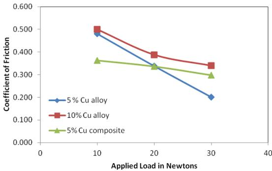
Figure 11 Coefficient of friction versus load of alloys and composite
