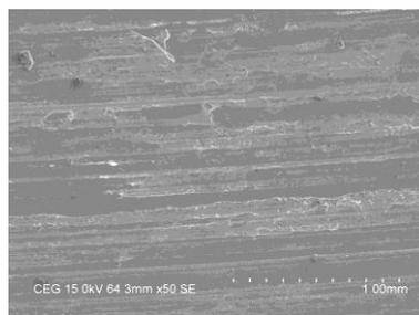
Figure 16 SEM image of worn out pin of Al-10-wt% Cu alloy at 20 N load, 3 m/sec sliding velocity and 1500 m sliding distance
