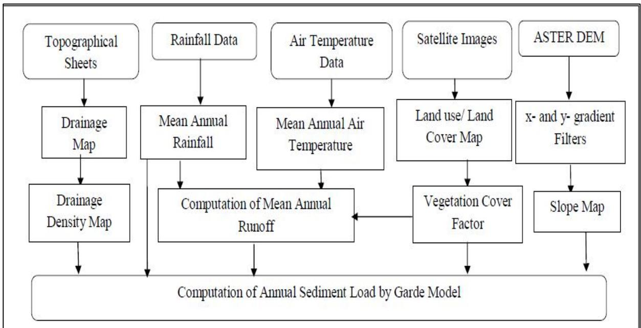
Figure 2 Flowchart illustrating procedure for quantification of sediment yield by Garde Model
