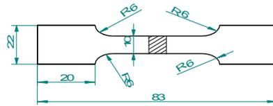
Fig 8: Tensile specimen prepared as per ASTM
