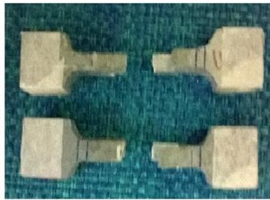
Fig 10 Photographic view of the broken tensile specimens
