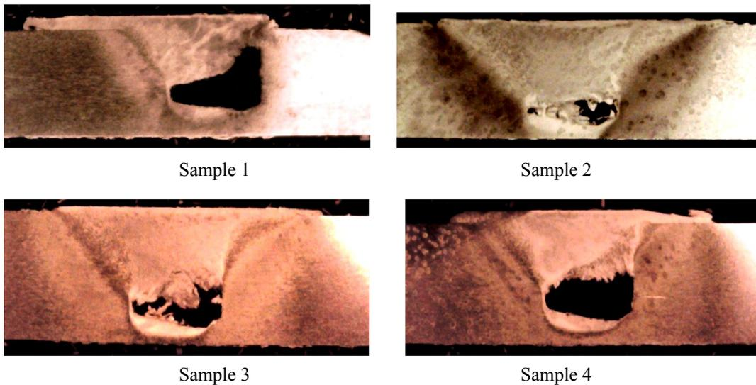
Fig 5: Macro structure of the Specimens showing varying sizes of tunnel defect
