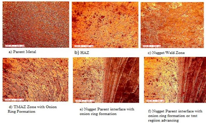
Fig 6 : Microimages of the Aluminum 2024 alloy
