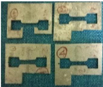
Fig 9: Photographic view of the cut portion of the Aluminium 2024 alloys
