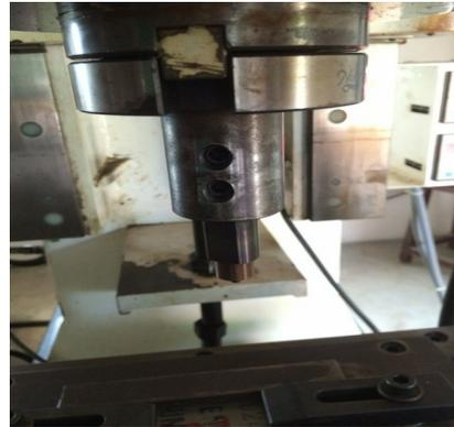
Fig 2: Photographic of Al 2024 alloy fixed in the FSW machine
