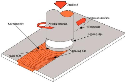
Fig 1 : Schematic diagram of the FSW process [1]
