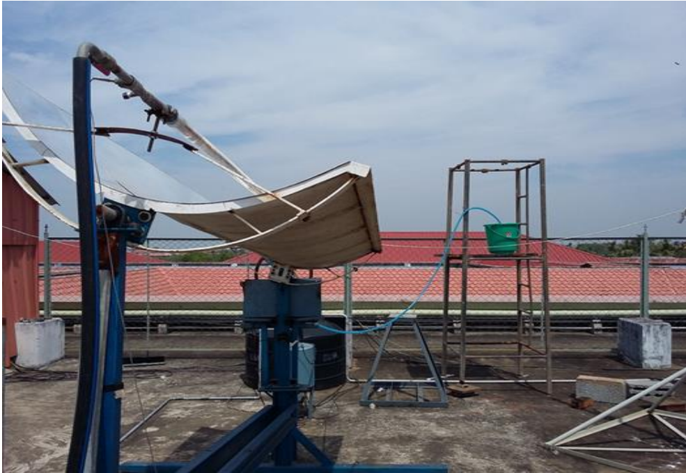
Fig.3 Experiment setup of Desalination system
