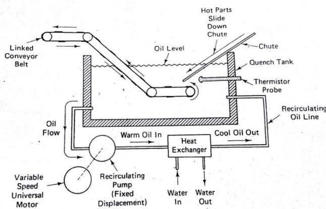
°Fig.1 Physical Layout of Quench oil Temperature control
