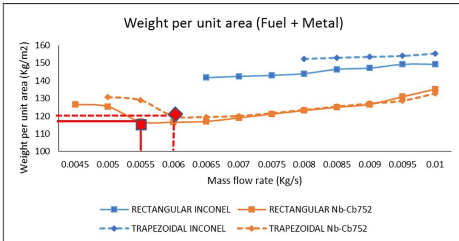
Fig. 3. Overall Weight per Unit Area Vs Mass Flow Rate
