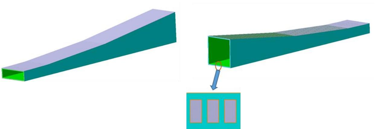
Fig. 5. Combustion Chamber with optimized cooling channel
