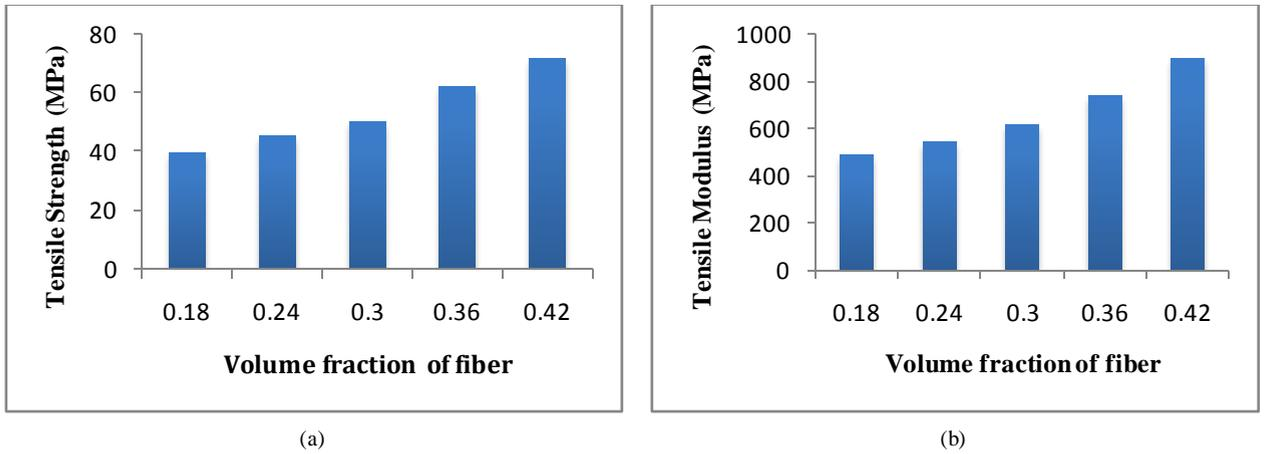
Fig. 2. Variation of (a) tensile strength (b) tensile modulus of composite with volume fraction of fibre.
