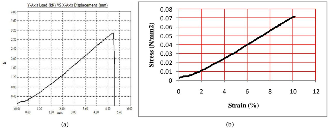
Fig. 3. (a) Load - Displacement curve (b) Stress - Strain curve of composite at volume fraction (0.42) of fiber.
