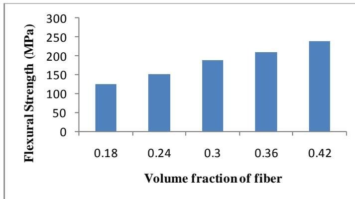
Fig. 4. Variation of flexural strength of composite with volume fraction of fibre.
