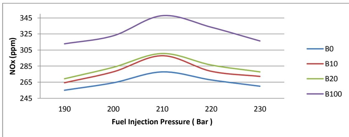
Figure 7 Variation of NO<sub>x</sub> Emission with fuel injection pressure
