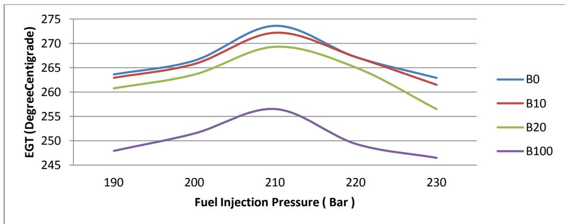
Figure 6 Variation of EGT with fuel injection pressure
