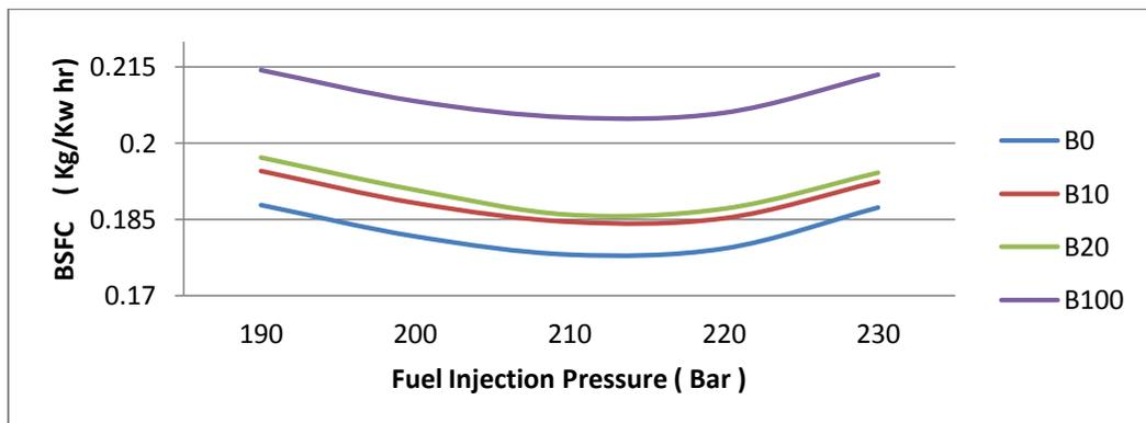
Figure 3 Variation of BSFC with fuel injection pressure
