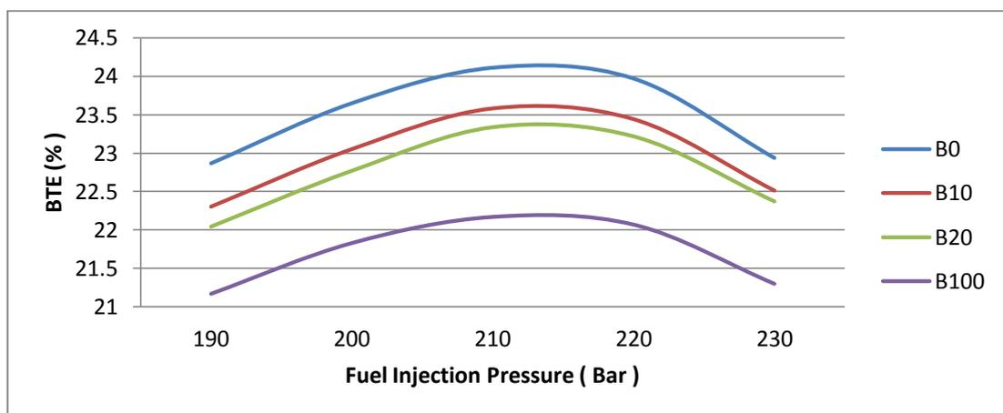
Figure 5 Variation of BTE with fuel injection pressure
