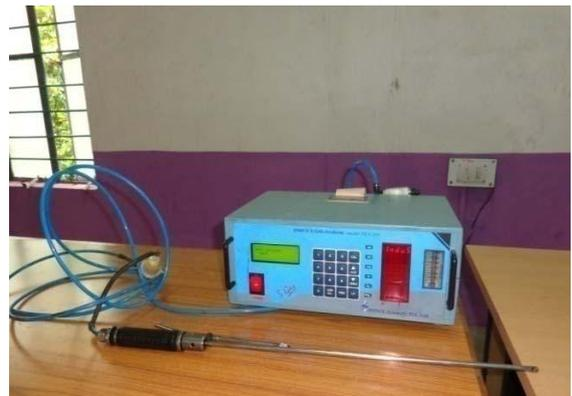
Figure 2 Exhaust Gas analyser
