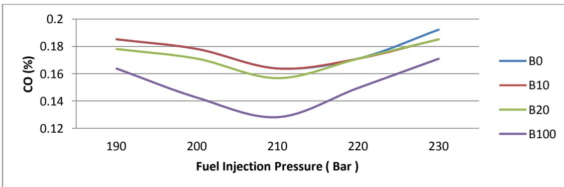
Figure 9 Variation of CO Emission with fuel injection pressure
