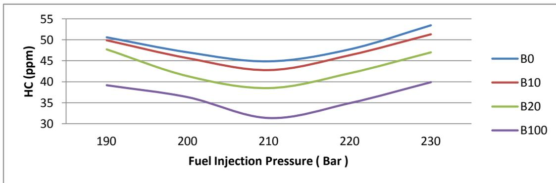
Figure 8 Variation of HC Emission with fuel injection pressure
