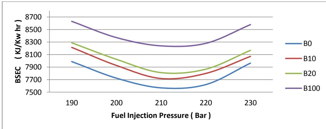
Figure 4 Variation of BSEC with fuel injection pressure
