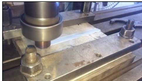
Fig. 2. Interaction between tool and base plate and experimentation on vertical milling head
