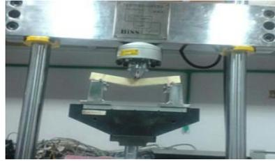
Fig.3.(b) 3-point bending test setup
