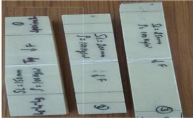
Fig.3.(a) Sandwich beam specimens
