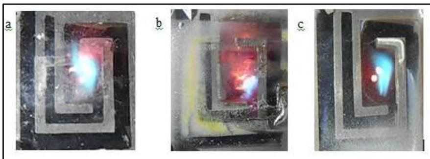
Fig. 2. Stable flames were observed at center of the one turn Swiss roll combustors for different materials at 20 mm depth (a) Stainless steel; (b) Aluminum; (c) Brass
