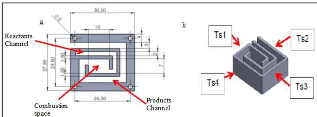
Fig. 1. Model of one turn Swiss roll combustor (a) dimensional details of channels and combustion space; (b) surface temperatures on surfaces 1 through 4 in sequence [2]
