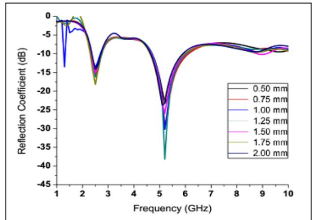
Fig. 5. Variation in reflection coefficient with L1.
