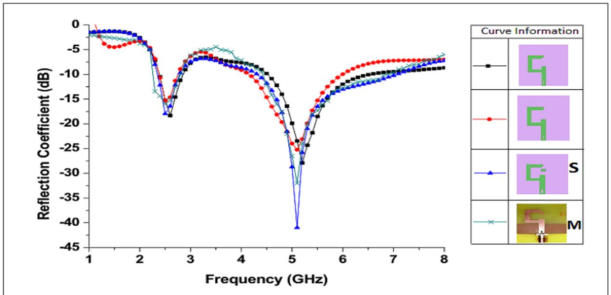
Fig. 2. Comparison between reflection coefficient results of the antenna at different stages.
