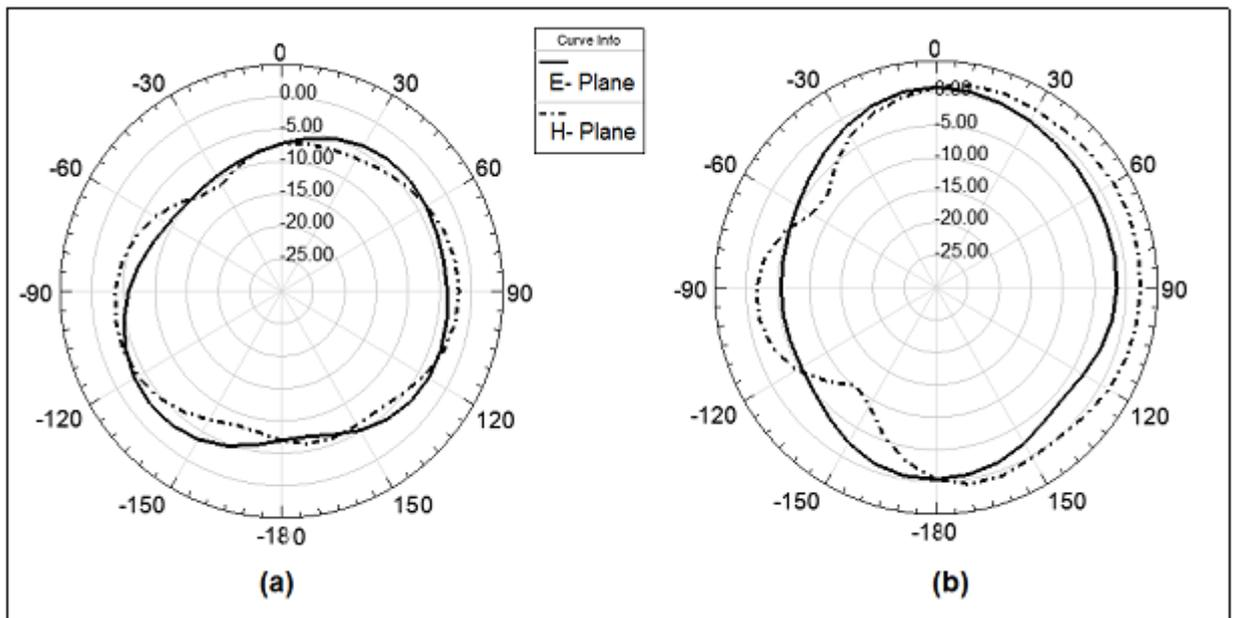
Fig. 3. E- Plane and H-Plane Simulated Radiation Pattern of proposed antenna at (a) 2.5 GHz (b) 5.15 GHz.
