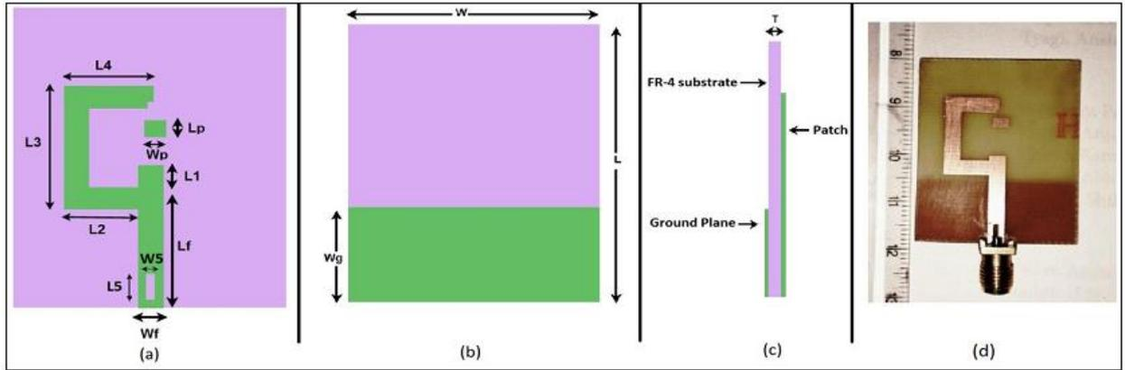
Fig. 1. Geometrical views of the antenna (a) Front view (b) Back view (c) Side view (d) Photograph of fabricated antenna.
