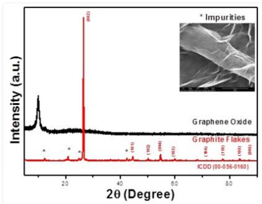
Fig. 1. XRD of GO thin film. The corresponding data for starting graphite flakes is shown in red.
