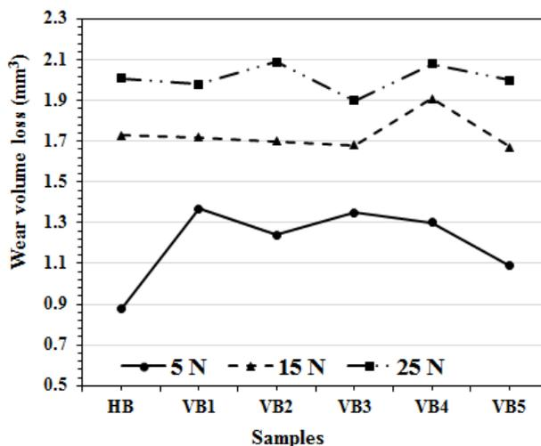
Fig. 4. Wear performance of horizontal and vertical built specimens at different loads.
