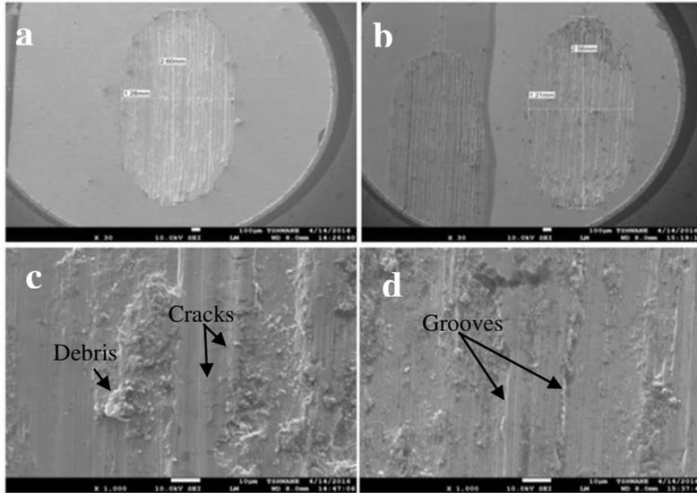
Fig. 5 - Wear track of HB and VB 3 specimens at 25N load (a, b) Lower magnification (c, d) Higher magnification.
