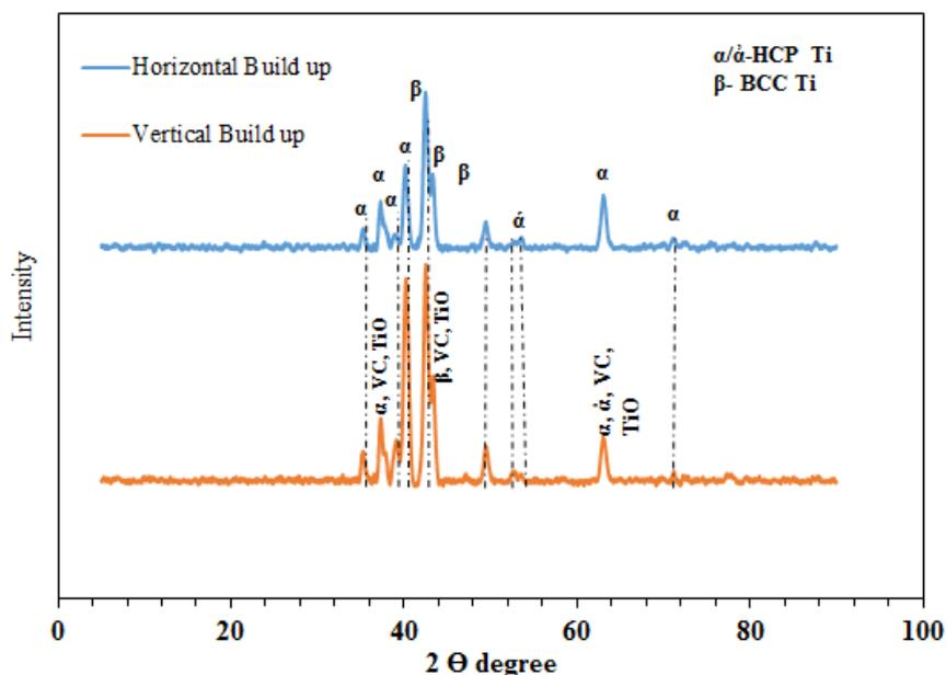
Fig. 3. XRD plots of horizontal and vertical built as-sintered specimens.
