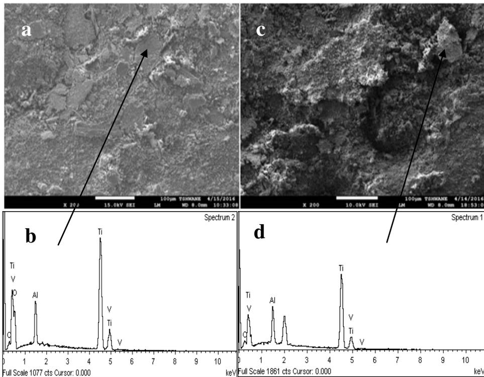
Fig. 6. (a, b) Wear debris and EDS of HB; (c, d) VB specimens at 25 N load.
