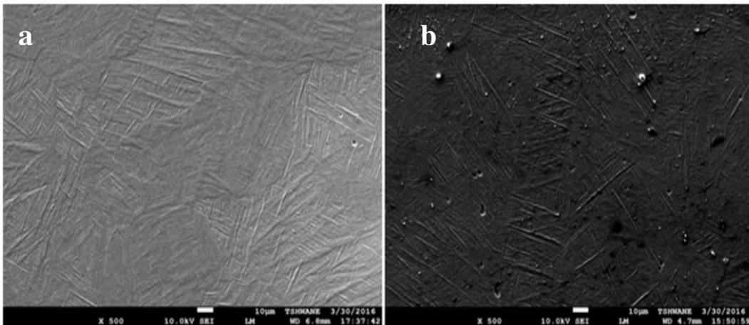
Fig. 2. (a) SEM images of HB; (b) SEM images of VB3 as-sintered specimens.
