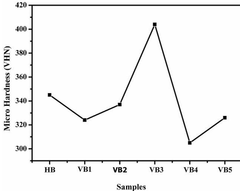
Fig. 1. Microhardness of horizontal and vertical built specimens
